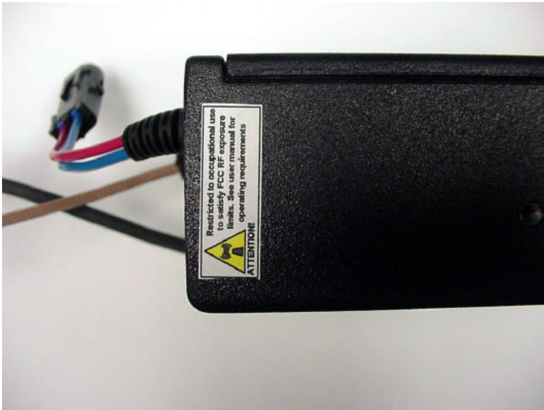
Radio side showing RF safety label
