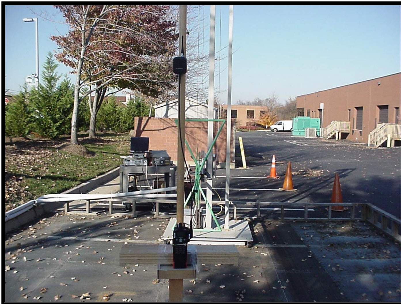
PHOTOGRAPH 1: RADIATED EMISSIONS FRONT VIEW (ANTENNA MOUNTED ON HANDSET)
