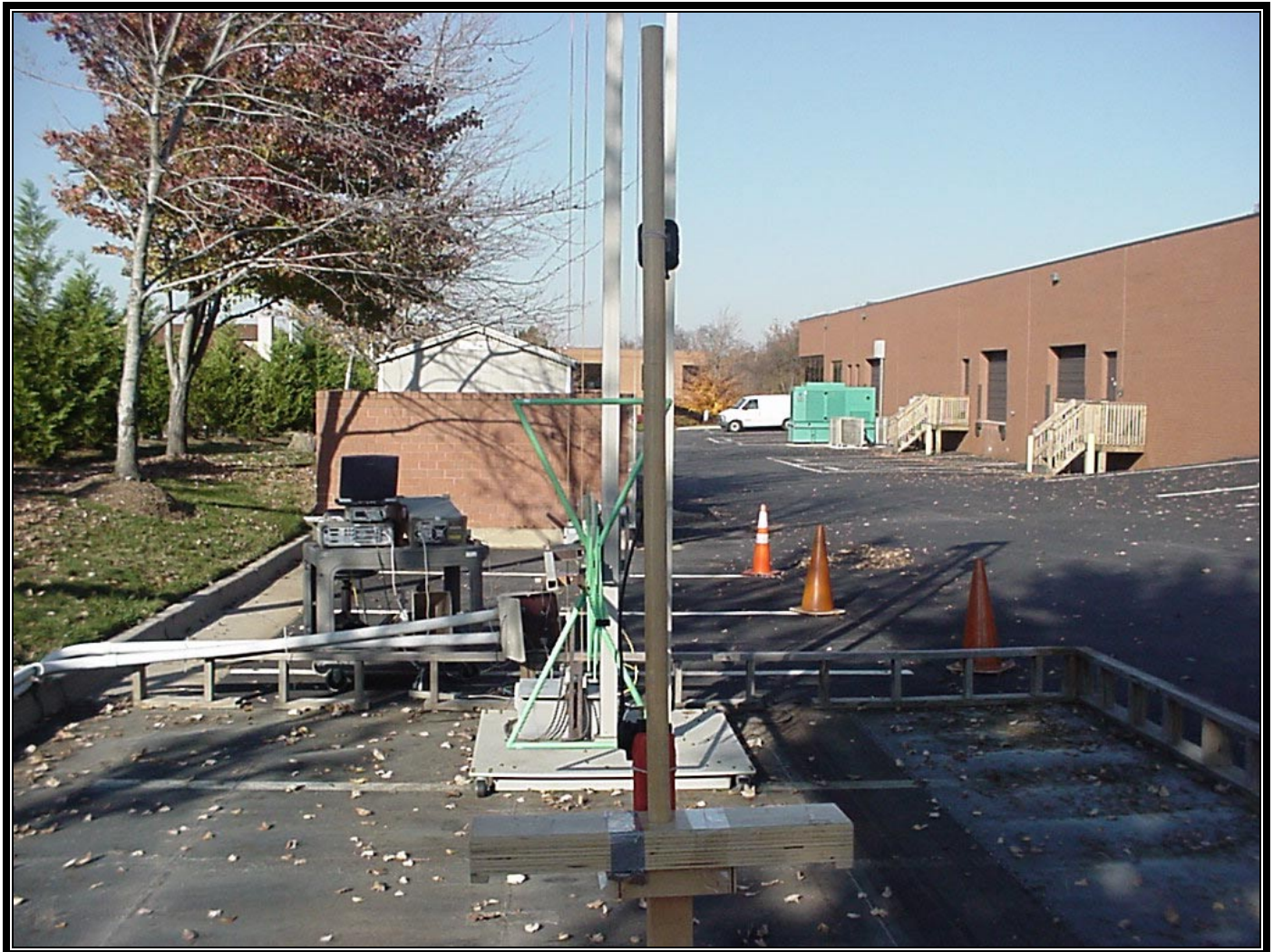
PHOTOGRAPH 2: RADIATED EMISSIONS REAR VIEW (ANTENNA MOUNTED ON HANDSET)
