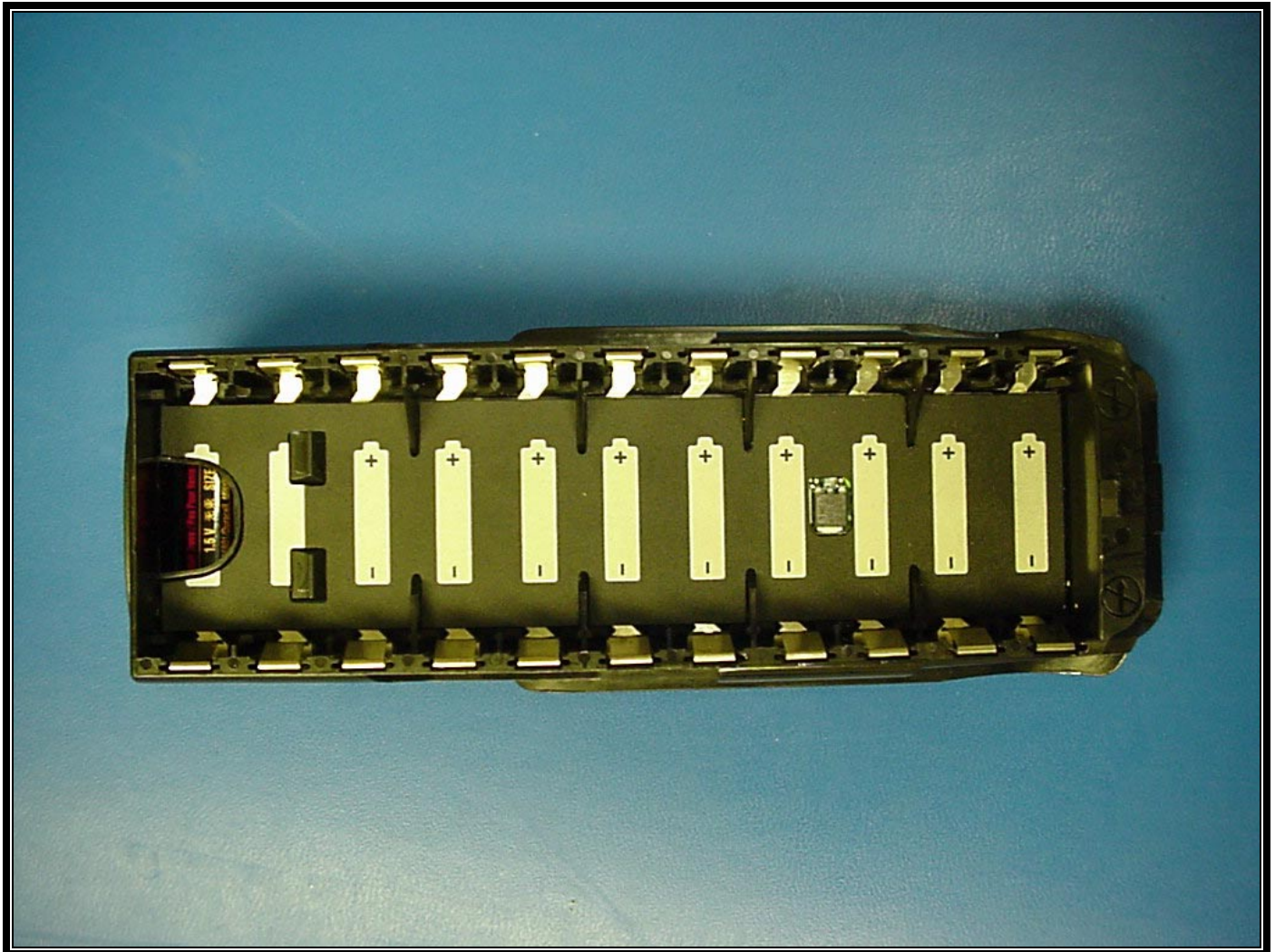
PHOTOGRAPH 8: FRONT VIEW OF BATTERY PACK (CELLS REMOVED)
