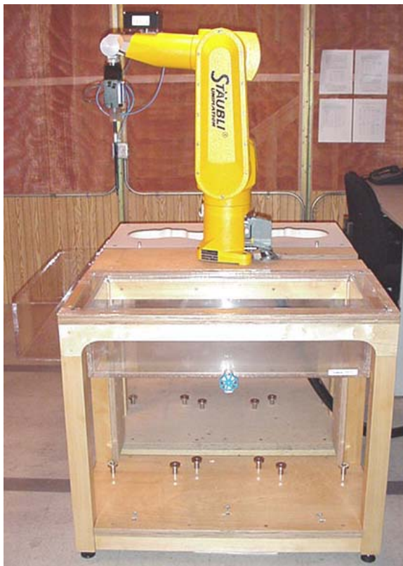
DASY4 SAR Measurement System with Plexiglas validation phantom
