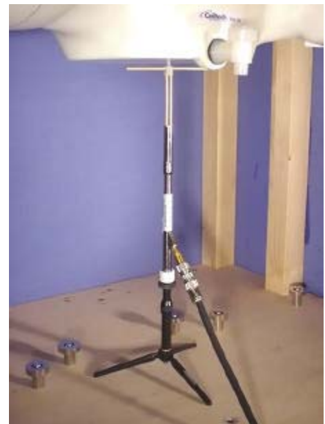
900MHz System Check Setup
