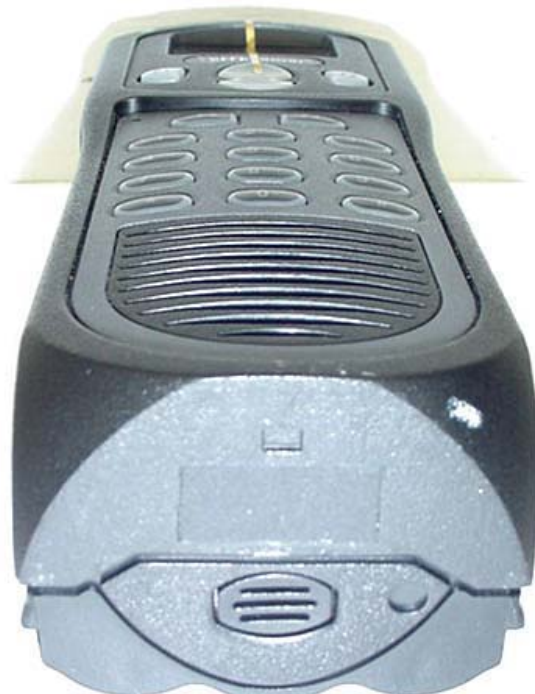
Bottom of DUT with NiMH Battery Pack
