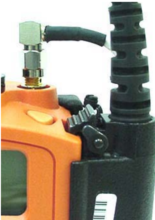
Front View of Antenna Termination
