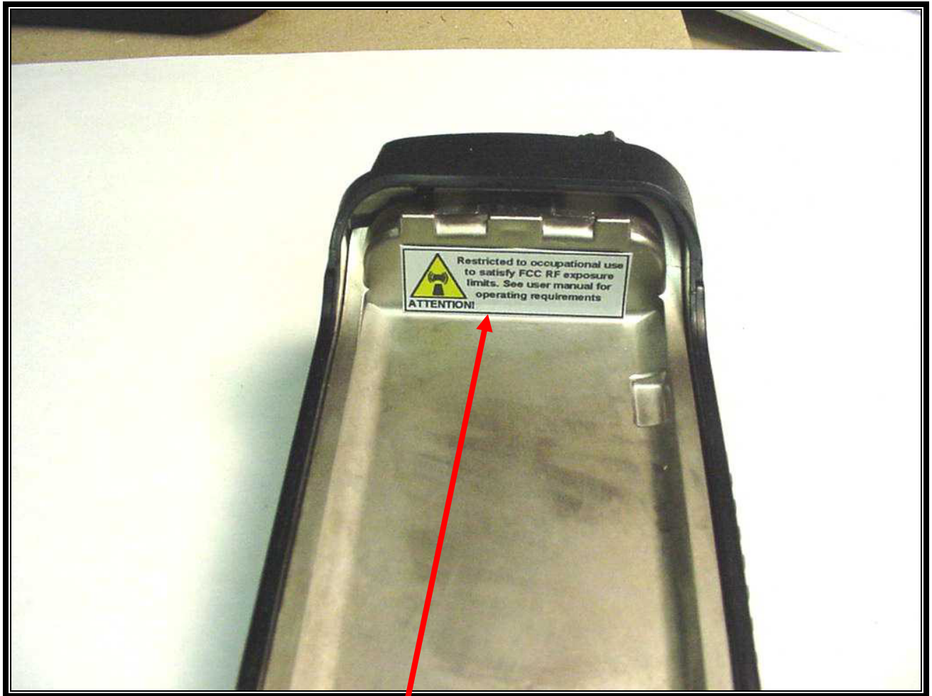
PHOTOGRAPH 2: RF WARNING LABEL & LOCATION
