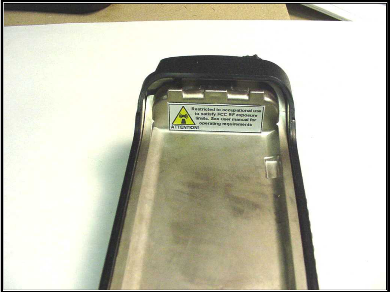
PHOTOGRAPH 2: RF WARNING LABEL
