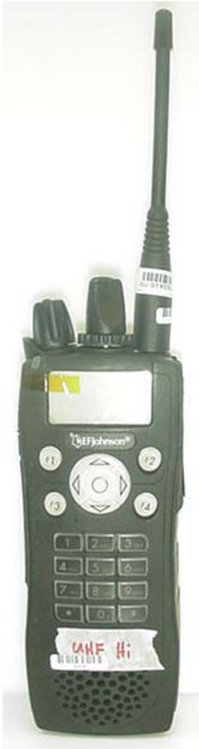
Front of Radio with 1/4-Wave Whip Antenna
