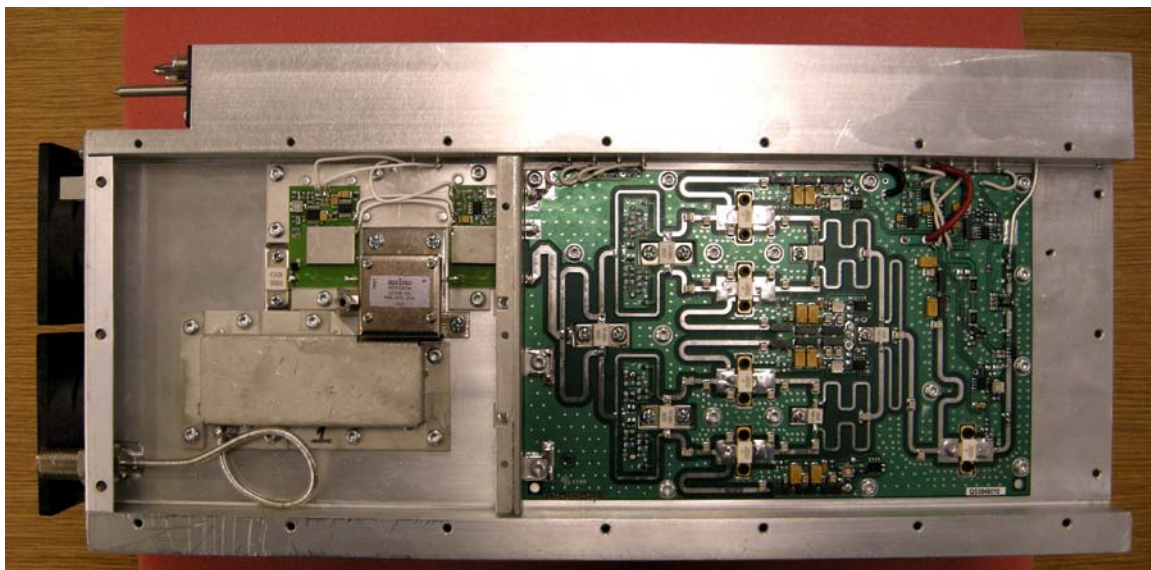
PA Board, Low Pass Filter, and RF Detector in Chassis
