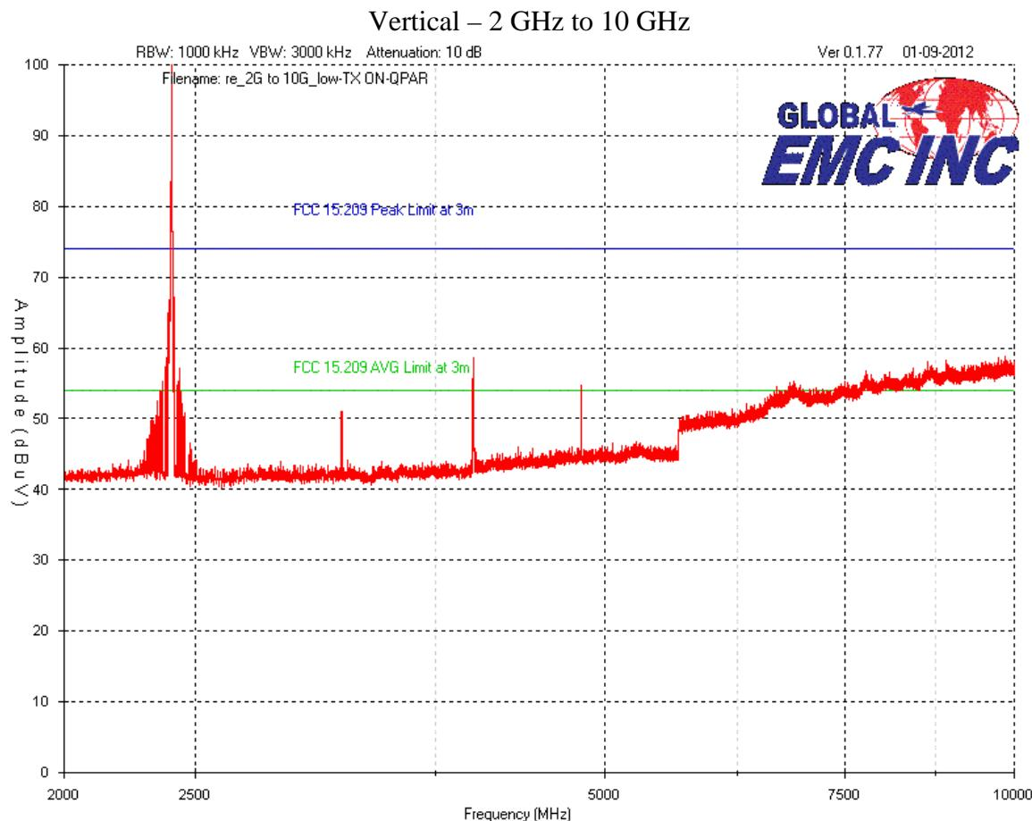
The above graph represents low channel (channel 1) as representative of peak digital modulated emissions. See table for final maximized peak/average measurements.
