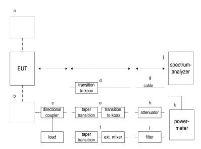
Setup 1.2 x...x: conducted emissions in test lab
