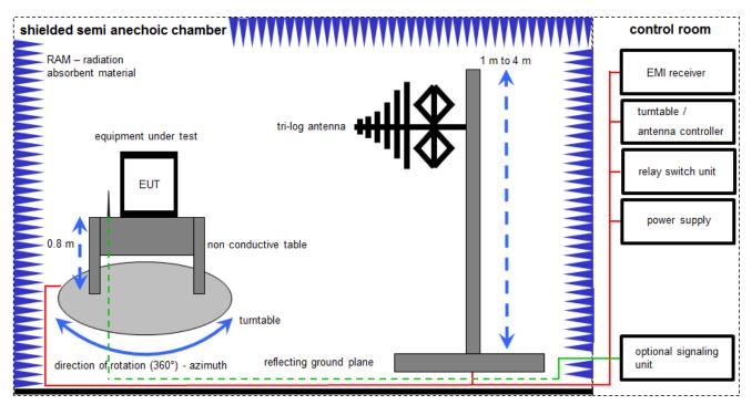
Measurement distance: tri-log antenna 10 meter
