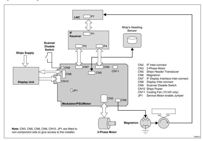
Figure 4. Scanner Interfaces
