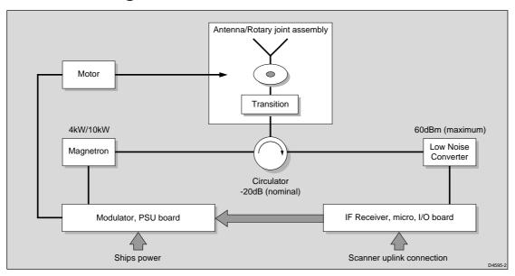
Figure 1. Scanner Block Diagram
