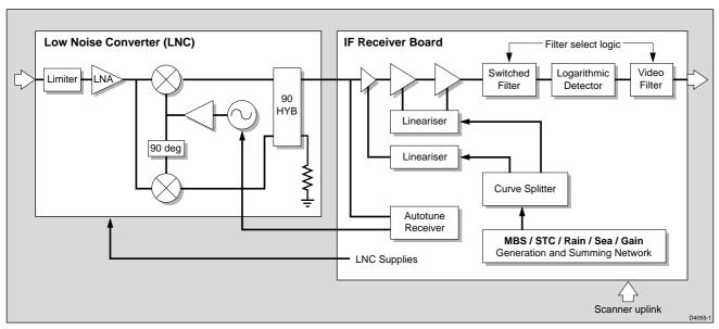
Figure 2. Receiver Configuration (LNC/IF)
