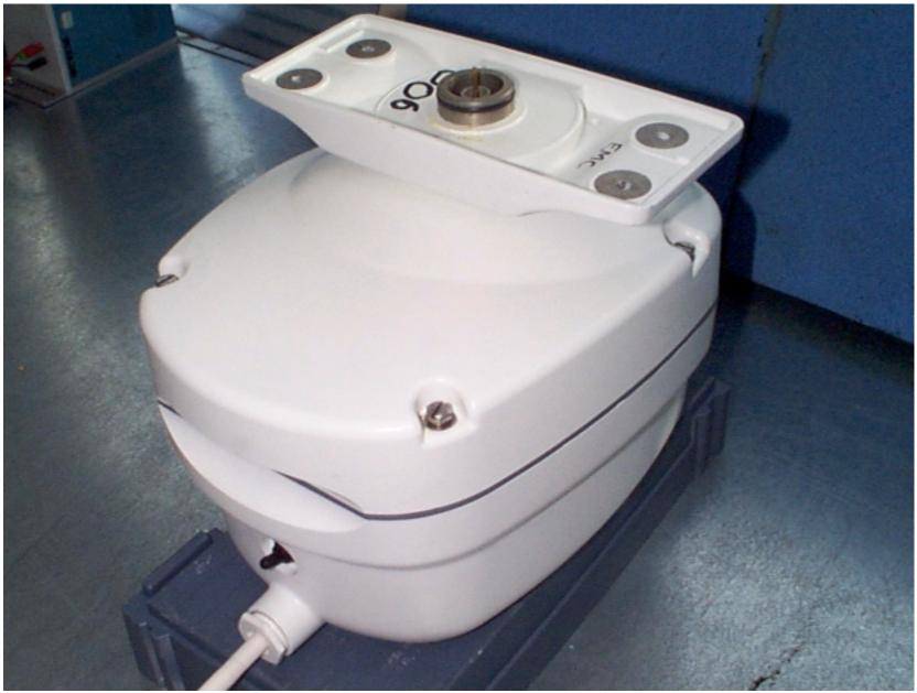
10kW, 48" Open Array Scanner Unit 10kW Pedestal and 48" Array
