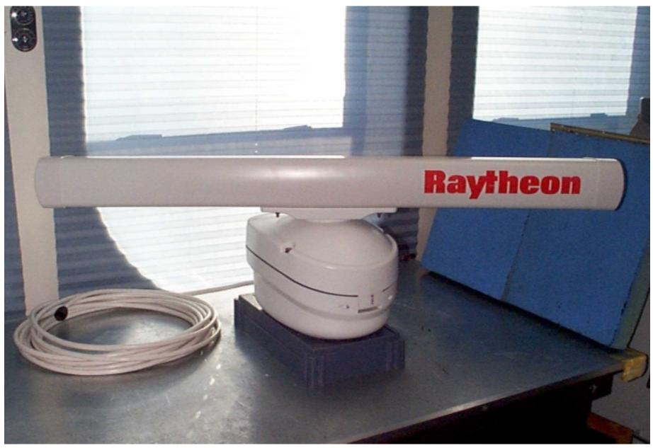
10kW, 48" Open Array Scanner Unit 10kW Pedestal and 48" Array
