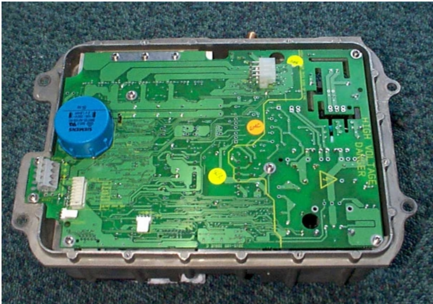
4kW, 48" Open Array Scanner unit 4kW Modulator/PSU PCB with screening plate removed
