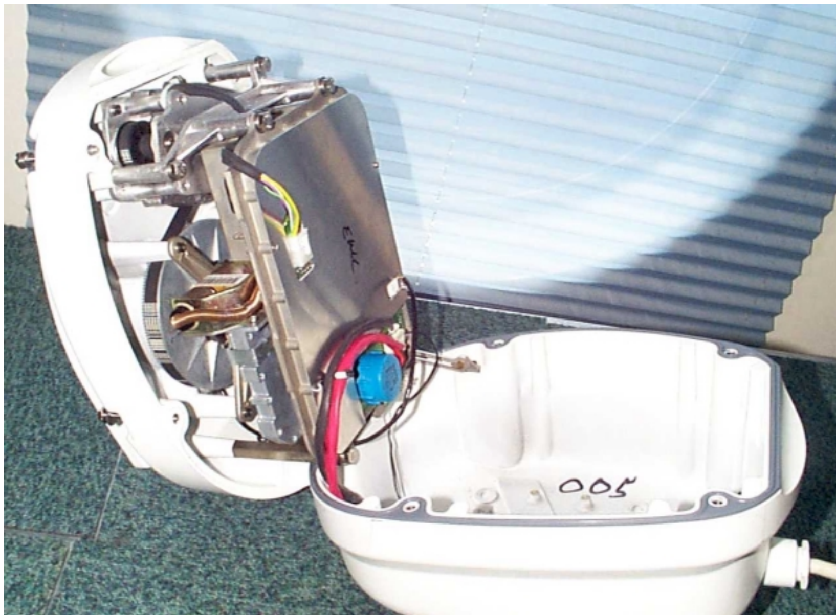
4kW, 48" Open Array Scanner Unit Pedestal open showing core assembly and gearbox
