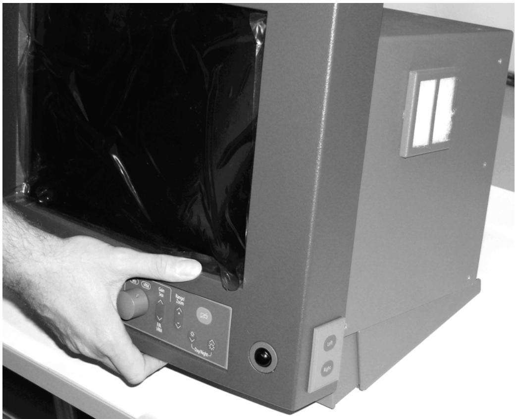
Figure: 1–5 Slide the NSC 18 Display into the lower base frame
