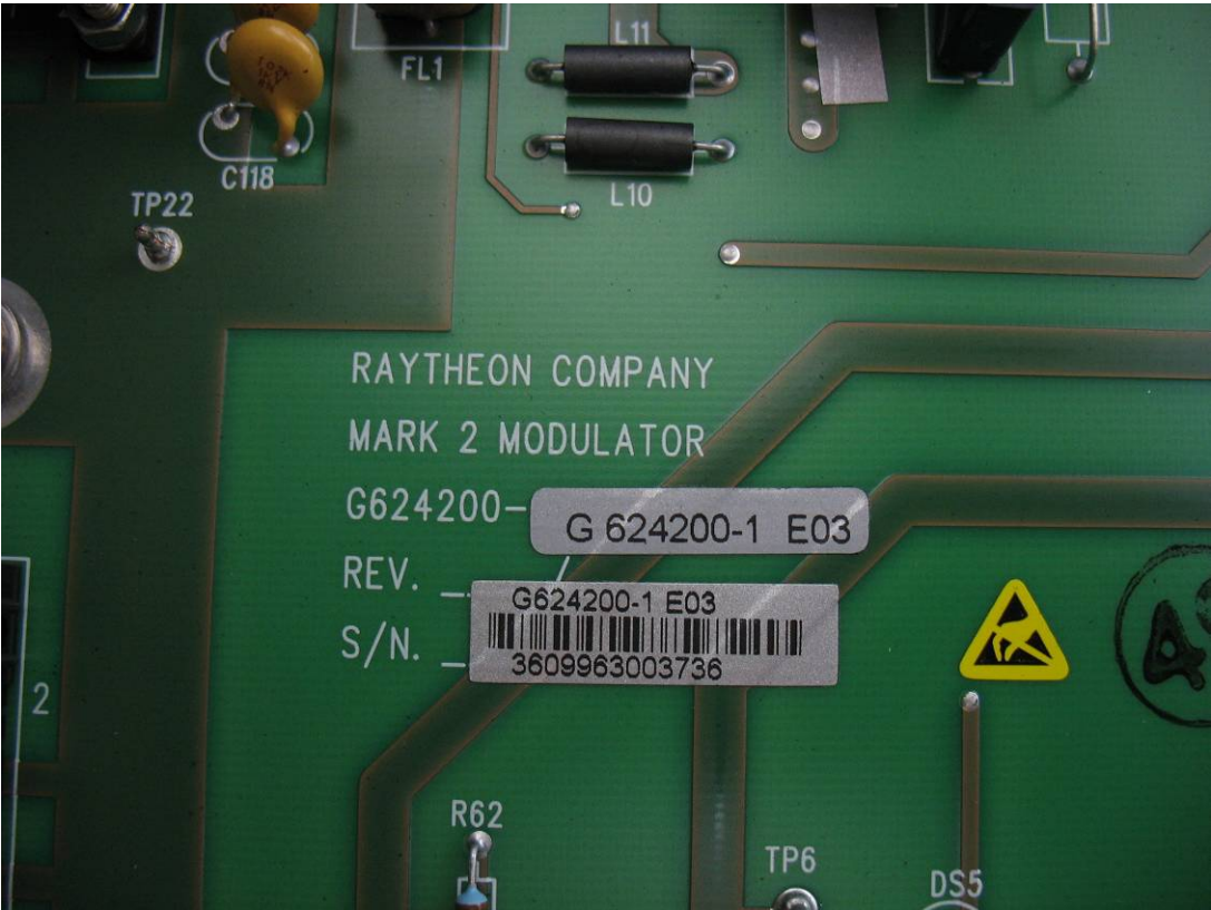
Photo No. 3: Modulator board
