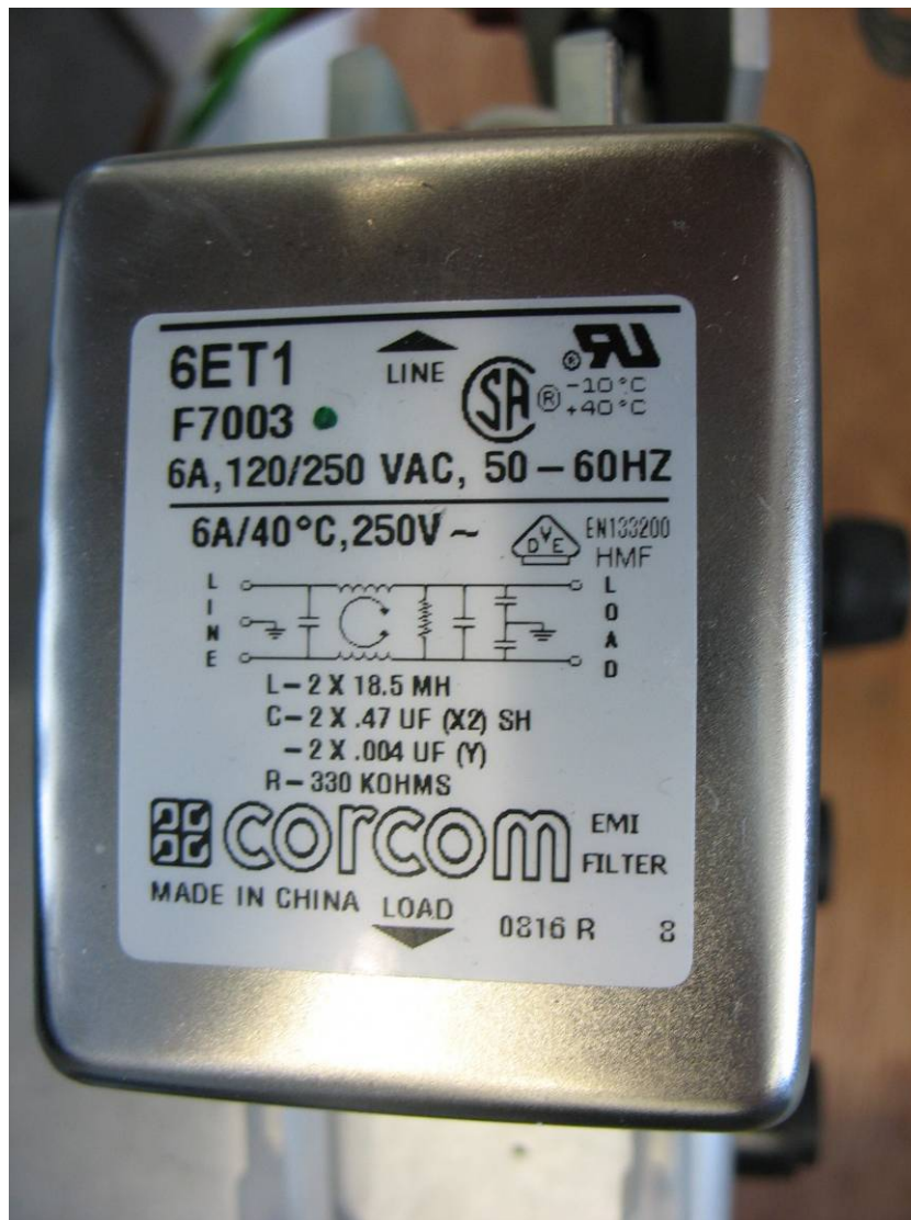
Photo No. 12: AC mains filter
