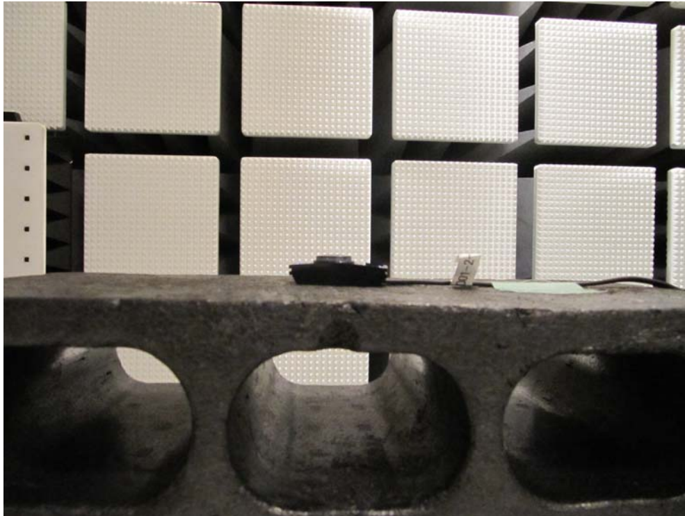
Photograph 6: Set-up for Radiated Emission, EUT Configuration X-Axis
