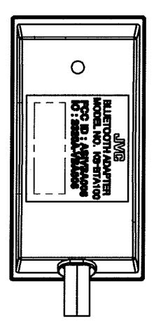
Label-A is located backside of bottom enclosure
