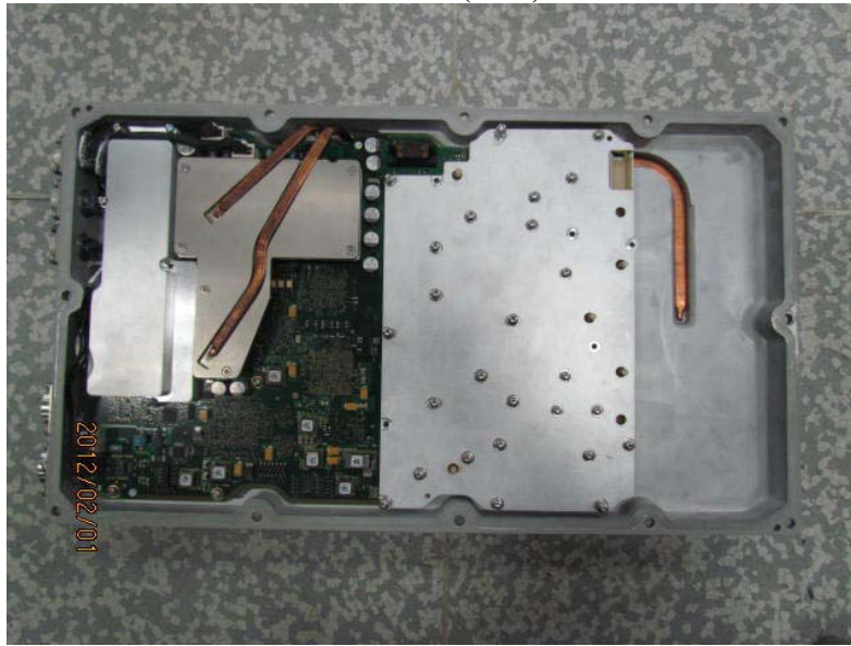
TRANSCIEVER (TRX) - TOP with COVERS REMOVED
