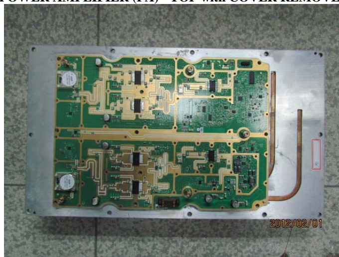
POWER AMPLIFIER (PA) - TOP with COVER REMOVED
