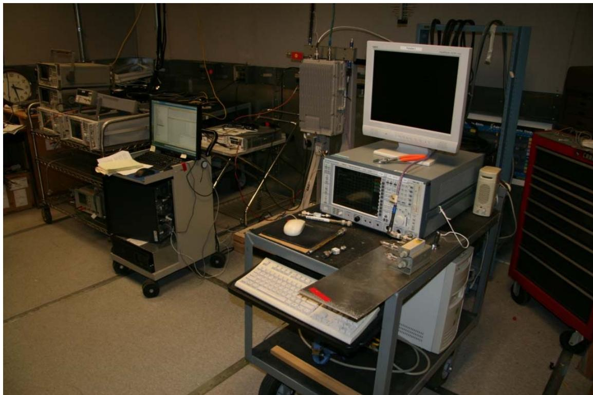
**TEST: Measurement of Radiated Spurious Emissions**
