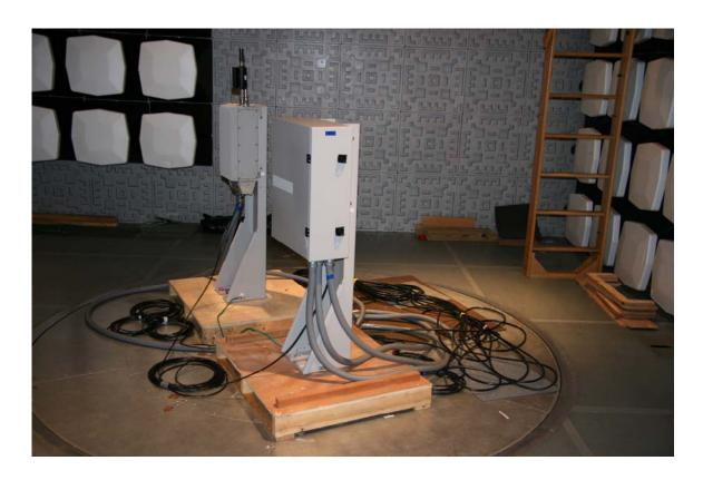
**TEST:** Measurement of Radiated Spurious Emissions
