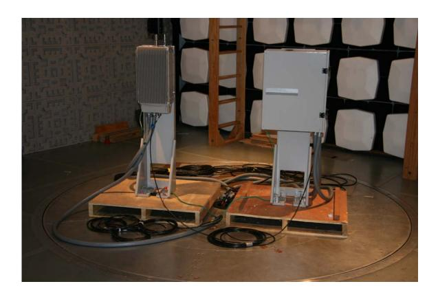
**TEST:** Measurement of Radiated Spurious Emissions
