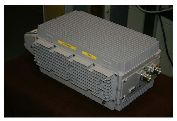
The 9341 RRH 60W 1900MHz RF Remote Radio Head (RRH) Front, Right Side and Top View .
