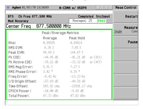
Modulation Characteristics: UARFCN Channel Number 1062 @ 882.50 MHz Tx Antenna Terminal at +47.8 dBm per single 5 MHz carrier
