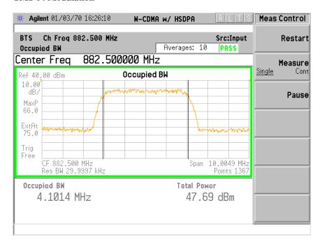
Carrier 99% Bandwidth Characteristics: UARFCN Channel Number 1107 @ 891.50 MHz Tx Antenna Terminal at +46 dBm per single 5 MHz carrier TM1-64 Modulation
