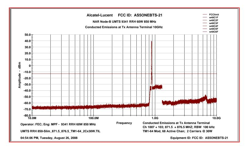
Two Carrier Conducted Emissions Characteristics: UARFCN Channel Number 1082 @ 886.50 MHz + CN 11107 @ 891.5 MHz Tx Antenna Terminal at +44.8 dBm per carrier TM1-64 Test Modulation
