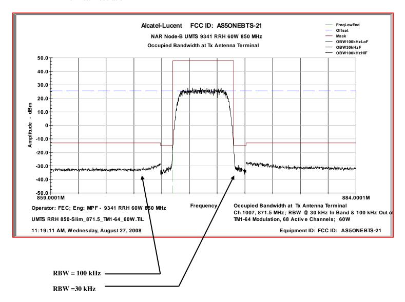
Occupied Bandwidth Characteristics: UARFCN Channel Number 1037 @ 877.50 MHz Tx Antenna Terminal at +47.8 dBm per single 5 MHz carrier TM1-64 Test Modulation
