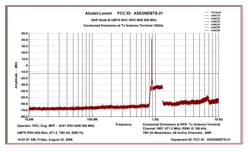
Conducted Emissions Characteristics: UARFCN Channel Number 1037 @ 877.50 MHz Tx Antenna Terminal at +47.8 dBm per single 5 MHz carrier TM1-64 Test Modulation
