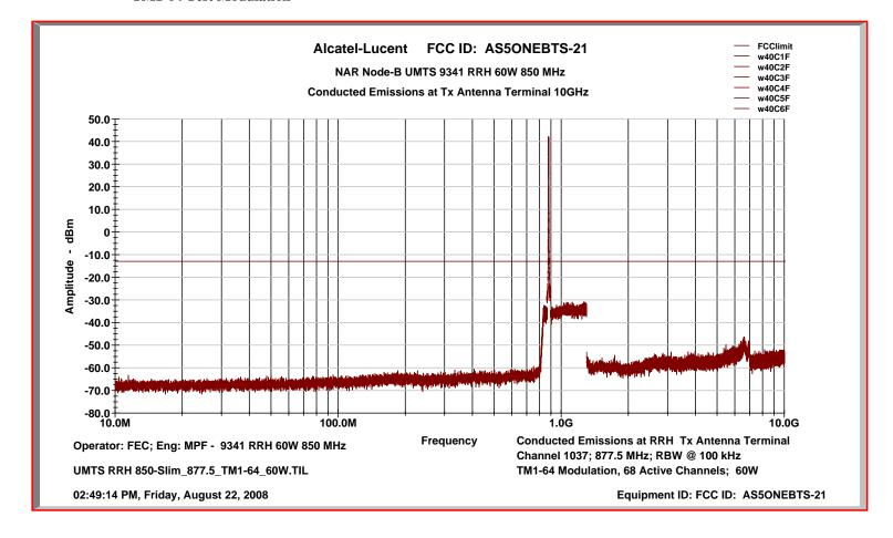
Conducted Emissions Characteristics: UARFCN Channel Number 1062 @ 882.50 MHz Tx Antenna Terminal at +47.8 dBm per single 5 MHz carrier TM1-64 Test Modulation
