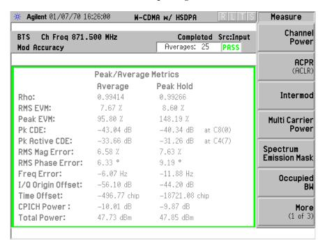
Modulation Characteristics: UARFCN Channel Number 1037 @ 877.50 MHz Tx Antenna Terminal at +47.8 dBm per single 5 MHz carrier
