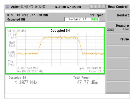
Carrier 99% Bandwidth Characteristics: UARFCN Channel Number 1062 @ 882.50 MHz Tx Antenna Terminal at +46 dBm per single 5 MHz carrier TM1-64 Modulation
