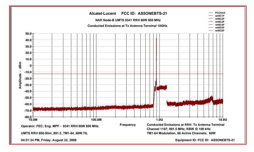
Two Carrier Conducted Emissions Characteristics: UARFCN Channel Number 1007 @ 871.50 MHz + CN 1032 @ 876.5 MHz Tx Antenna Terminal at +44.8 dBm per carrier TM1-64 Test Modulation
