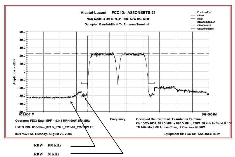
Two Carrier Occupied Bandwidth Characteristics: UARFCN Channel Number 1082 @ 886.50 MHz + CN 1107 @ 891.5 MHz Tx Antenna Terminal at +44.8 dBm per carrier TM1-64 Test Modulation
