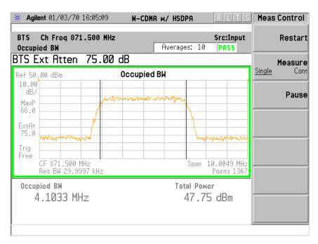
Carrier 99% Bandwidth Characteristics: UARFCN Channel Number 1037 @ 877.50 MHz Tx Antenna Terminal at +46 dBm per single 5 MHz carrier TM1-64 Modulation
