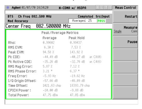
Modulation Characteristics: UARFCN Channel Number 1107 @ 891.50 MHz Tx Antenna Terminal at +47.8 dBm per single 5 MHz carrier
