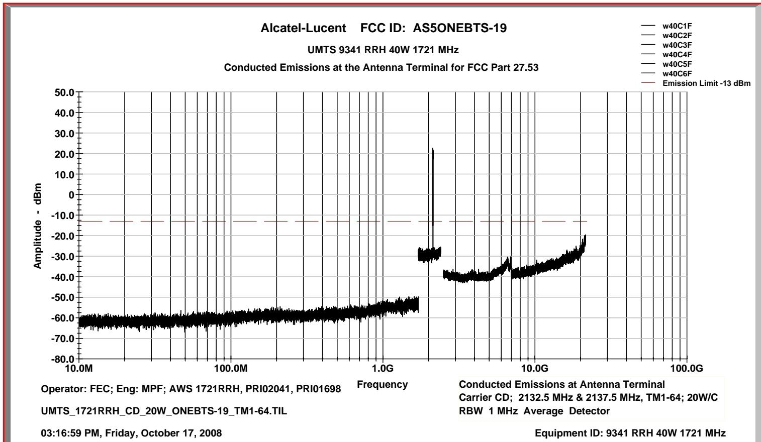
**Highest Settable Carrier Pair - F Block - TM1-64 Test Modulation**
