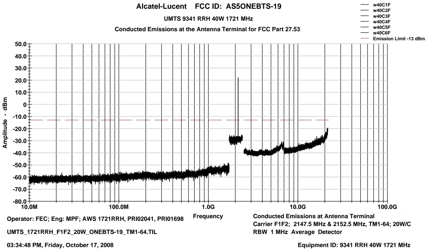
**PART 2.1051 MEASUREMENTS REQUIRED: SPURIOUS EMISSIONS AT THE ANTENNA TERMINALS – Three Carrier Operation**
