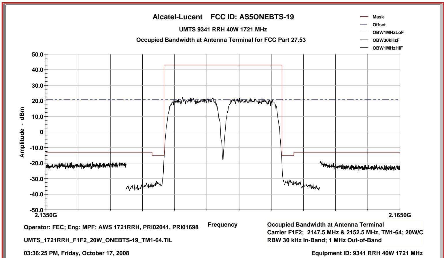
**PART 2.1049 MEASUREMENTS REQUIRED: OCCUPIED BANDWIDTH - THREE CARRIERS****- CONTINUED -**
