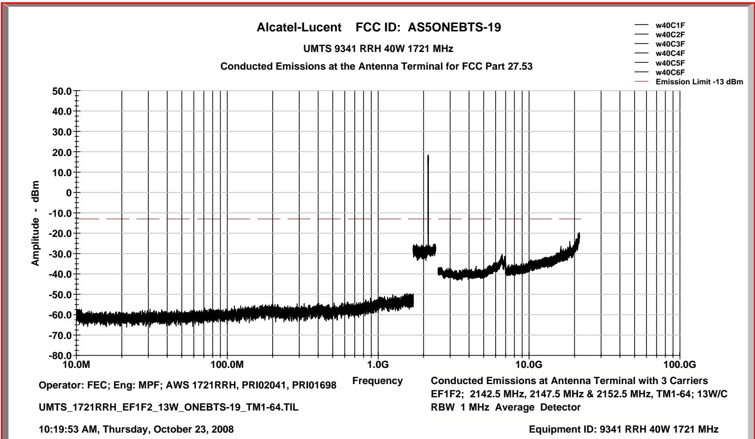
**PART 2.1053 MEASUREMENTS REQUIRED: FIELD STRENGTH OF SPURIOUS RADIATION**
