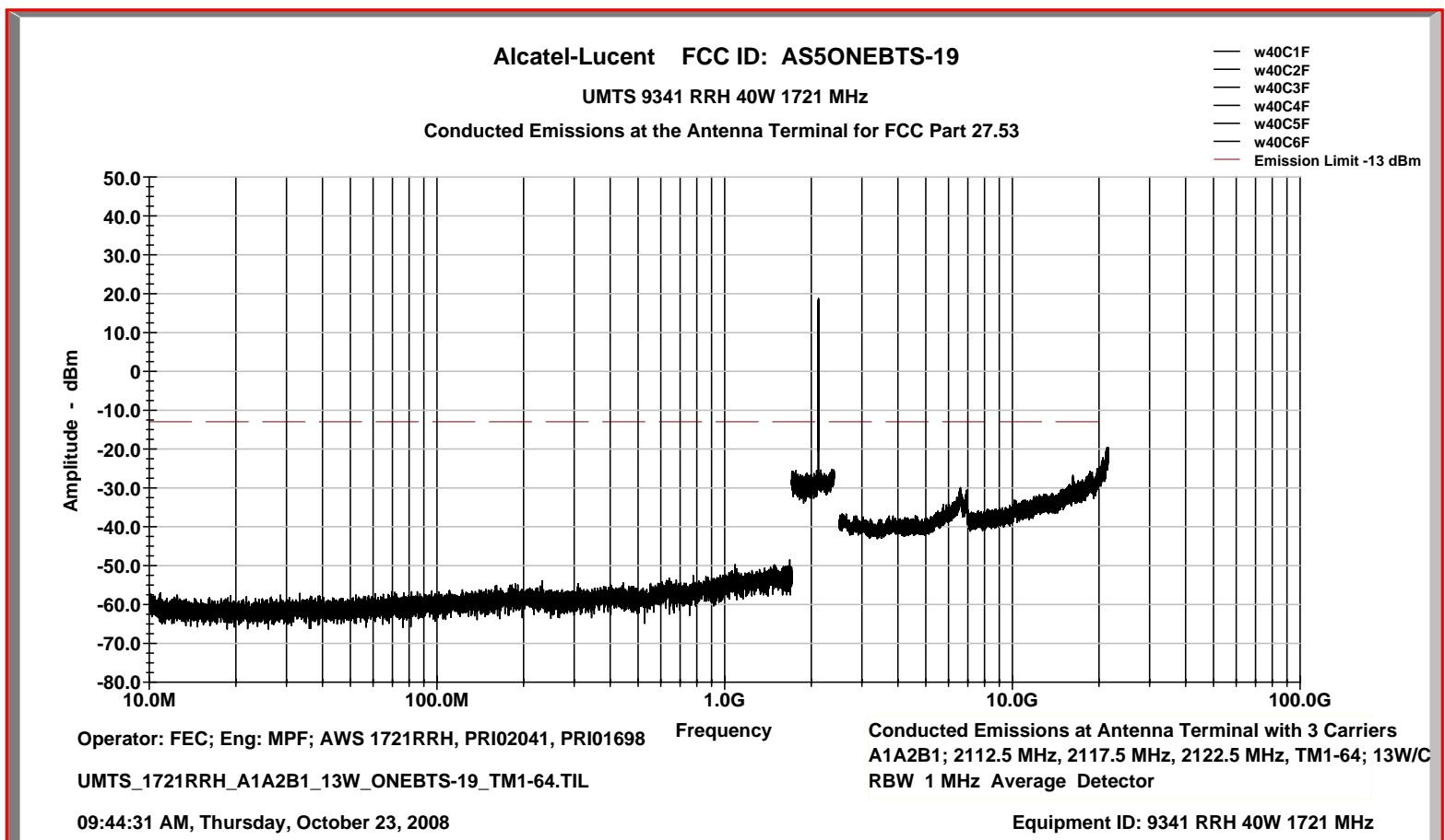
**Highest Settable 3 Adjacent Carriers - TM1-64 Test Modulation**
