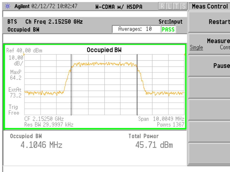
**PART 2.1049 MEASUREMENTS REQUIRED: OCCUPIED BANDWIDTH - SINGLE CARRIER****- CONTINUED -**
