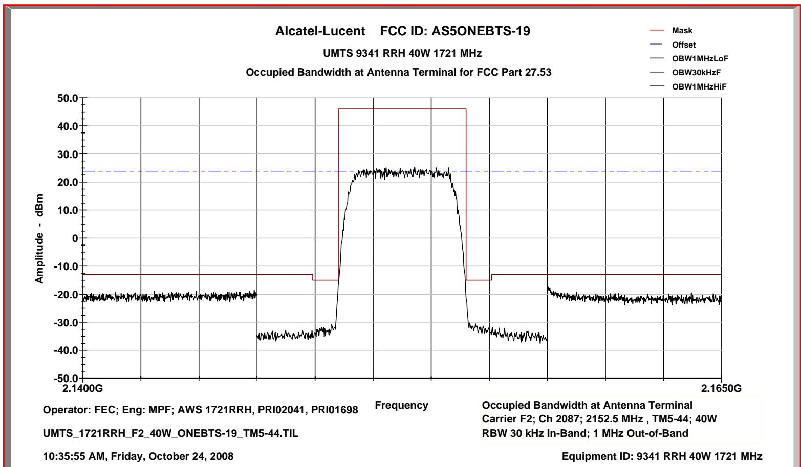
**PART 2.1049 MEASUREMENTS REQUIRED: OCCUPIED BANDWIDTH - TWO CARRIERS****- CONTINUED -**
