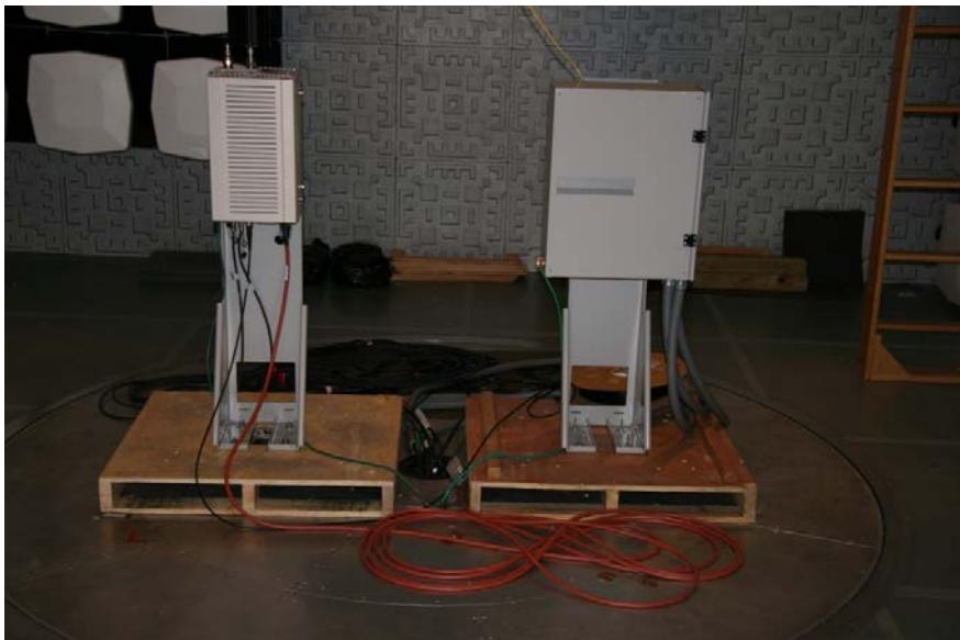
Test Set-Up for Measurement of Frequency Stability:
