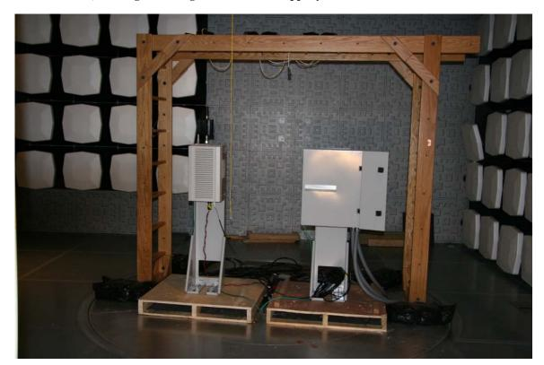
**TEST:** Measurement of Radiated Spurious Emissions
