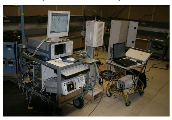
**TEST:** Measurement of RF Power Output
