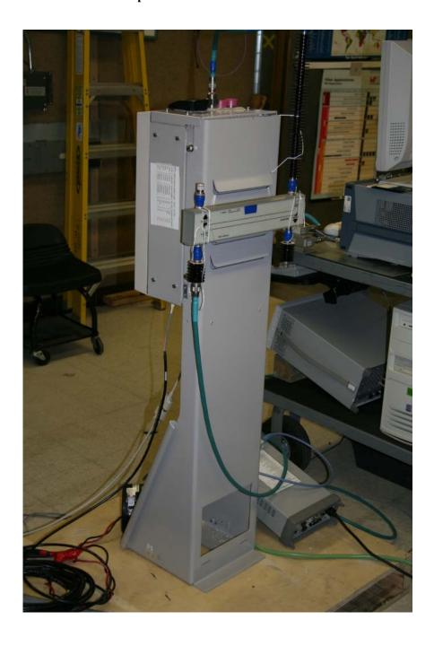
**TEST:** Measurement of Radiated Spurious Emissions
