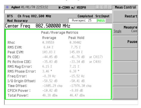
Modulation Characteristics: UARFCN Channel Number 1107 @ 891.50 MHz Tx Antenna Terminal at +46 dBm per single 5 MHz carrier
