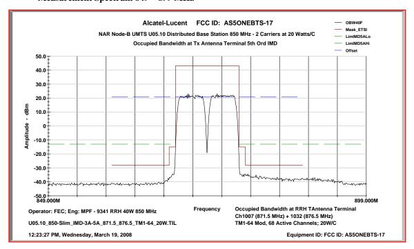
Pair #1, A-Band: Ch 1007, 871.5 MHz + Ch 1032, 876.5 MHz Measurement Spectrum 10 MHz - 10 GHz at Res BW 100 kHz
