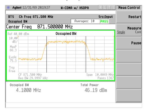
Carrier 99% Bandwidth Characteristics: UARFCN Channel Number 1037 @ 877.50 MHz Tx Antenna Terminal at +46 dBm per single 5 MHz carrier with TM1-64 Modulation
