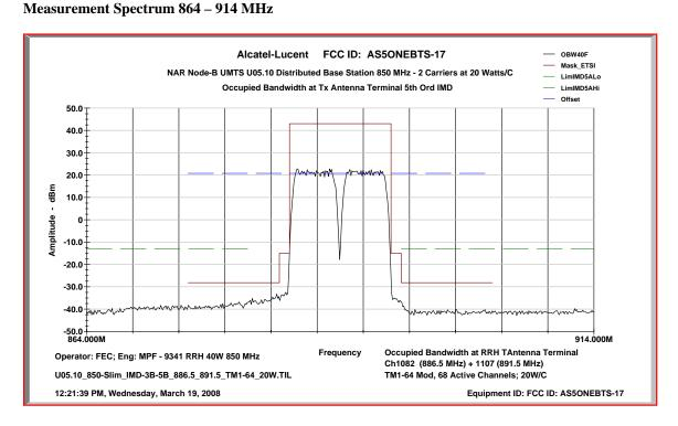
Pair #2, B-Band: Ch 1082, 886.5 MHz + Ch 1107, 891.5 MHz Measurement Spectrum 10 MHz – 10 GHz at Res BW 100 kHz
