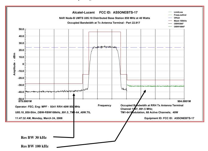
The ETSI TS 25.141 Emission Mask is designed based on a 30 kHz Res BW in-band.
