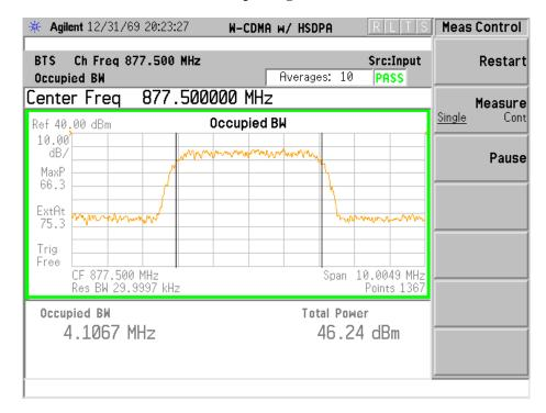
Carrier 99% Bandwidth Characteristics: UARFCN Channel Number 1062 @ 882.50 MHz Tx Antenna Terminal at +46 dBm per single 5 MHz carrier with TM1-64 Modulation
