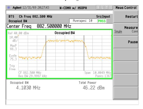
Carrier 99% Bandwidth Characteristics: UARFCN Channel Number 1107 @ 891.50 MHz Tx Antenna Terminal at +46 dBm per single 5 MHz carrier with TM1-64 Modulation
