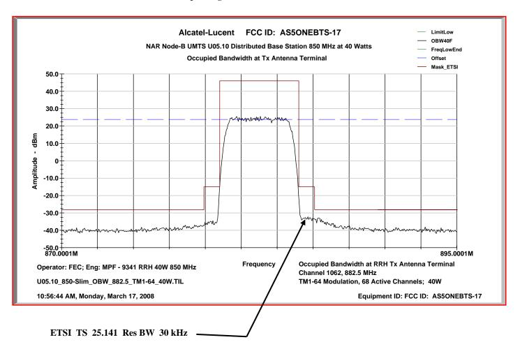
The ETSI TS 25.141 Emission Mask is designed based on a 30 kHz Res BW in-band.
