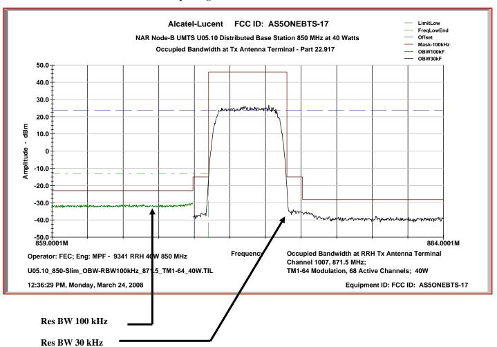
The ETSI TS 25.141 Emission Mask is designed based on a 30 kHz Res BW in-band.
