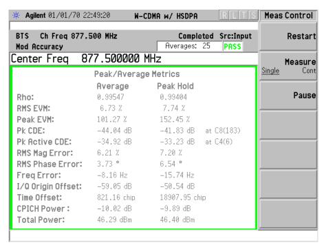
Modulation Characteristics: UARFCN Channel Number 1062 @ 882.50 MHz Tx Antenna Terminal at +46 dBm per single 5 MHz carrier
