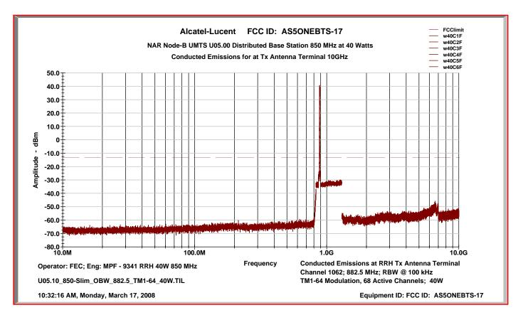
Conducted Emissions Characteristics: UARFCN Channel Number 1107 @ 891.50 MHz
