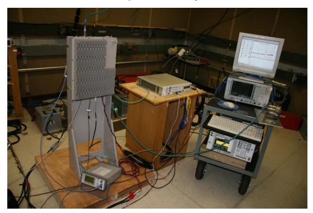
**TEST:** Measurement of RF Power Output
