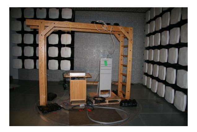
**TEST:** Measurement of Frequency Stability
