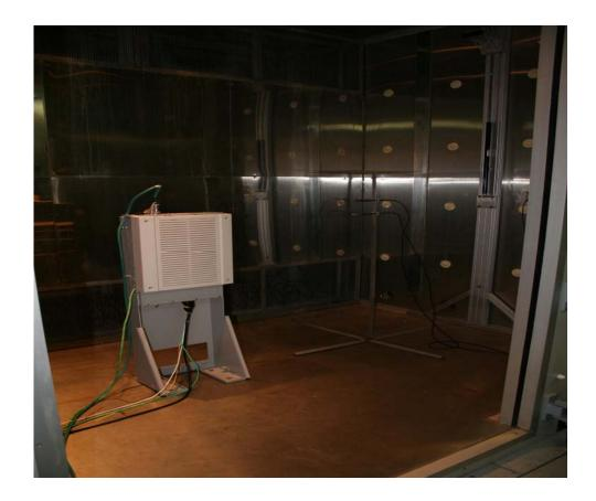
**TEST:** Measurement of Frequency Stability
