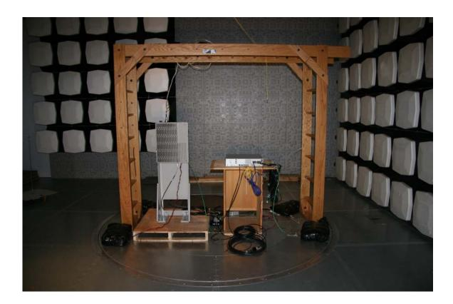
**TEST:** Measurement of Radiated Spurious Emissions
