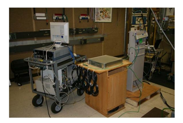
**TEST:** Measurement of Radiated Spurious Emissions
