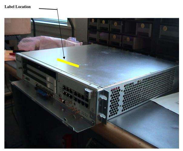
Top View of the Digital Base Band Unit Showing the Label Placement
