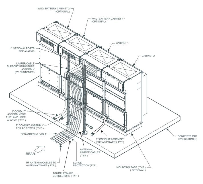
Modular Cell 4.0B primary and dual band cabinets with WNG24-BC battery cabinets installed on a rooftop Illustrated below is an outdoor site maximum 4.0B configuration, with primary and dual band Modular Cell 4.0B cabinets with WNG24-BC battery cabinets installed on a rooftop.
