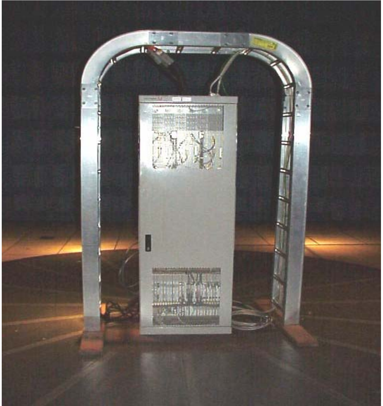
Lucent UMTS CDMA 850 Indoor Base Transceiver Station (BTS) Front View
