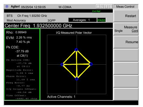
Modulation Characteristics: Frequency Block A; Carrier Channel A3 UMTS1900 Ch 62; 1942.5 MHz at Tx Antenna Terminal at +46 dBm per single 5 MHz carrier
