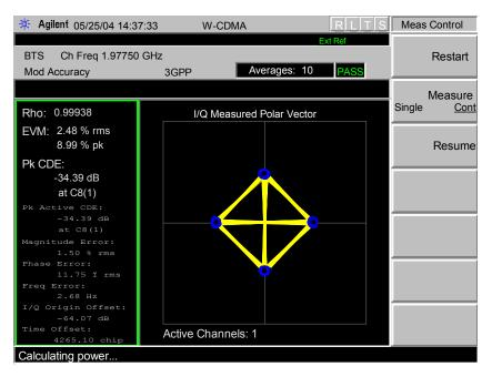
Modulation Characteristics: Frequency Block C, Carrier Channel C5 UMTS1900 Ch 287; 1987.5 MHz at Tx Antenna Terminal at +46 dBm per single 5 MHz carrier
