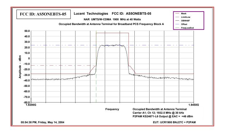
Occupied Bandwidth Characteristics Block A3 UMTS1900 Ch 62; 1942.5 MHz at Tx Antenna Terminal at +46 dBm per single 5 MHz carrier
