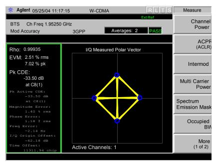
Modulation Characteristics: Frequency Block B, Carrier Channel B3 UMTS1900 Ch 162; 1962.5 MHz at Tx Antenna Terminal at +46 dBm per single 5 MHz carrier
