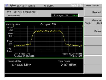
Carrier Bandwidth Characteristics: Frequency Block A; Carrier Channel A3 UMTS1900 Ch 62; 1942.5 MHz at Tx Antenna Terminal at +46 dBm per single 5 MHz carrier
