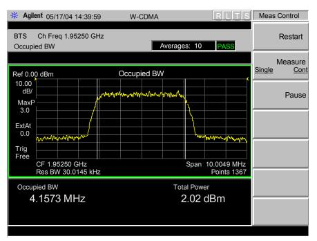
Carrier Bandwidth Characteristics: Frequency Block B, Carrier Channel B3 UMTS1900 Ch 162; 1962.5 MHz at Tx Antenna Terminal at +46 dBm per single 5 MHz carrier
