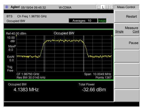
Carrier Bandwidth Characteristics: Frequency Block F, Carrier Channel F UMTS1900 Ch 212; 1972.5 MHz at Tx Antenna Terminal at +46 dBm per single 5 MHz carrier
