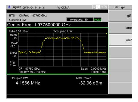
Carrier Bandwidth Characteristics: Frequency Block C, Carrier Channel C5 UMTS1900 Ch 287; 1987.5 MHz at Tx Antenna Terminal at +46 dBm per single 5 MHz carrier
