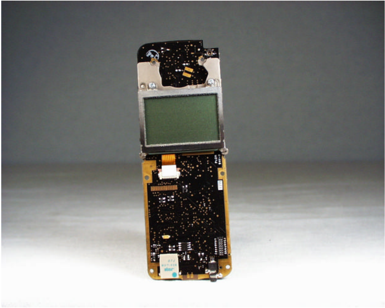
Component Side of PCB with LCD Display (Handset)
