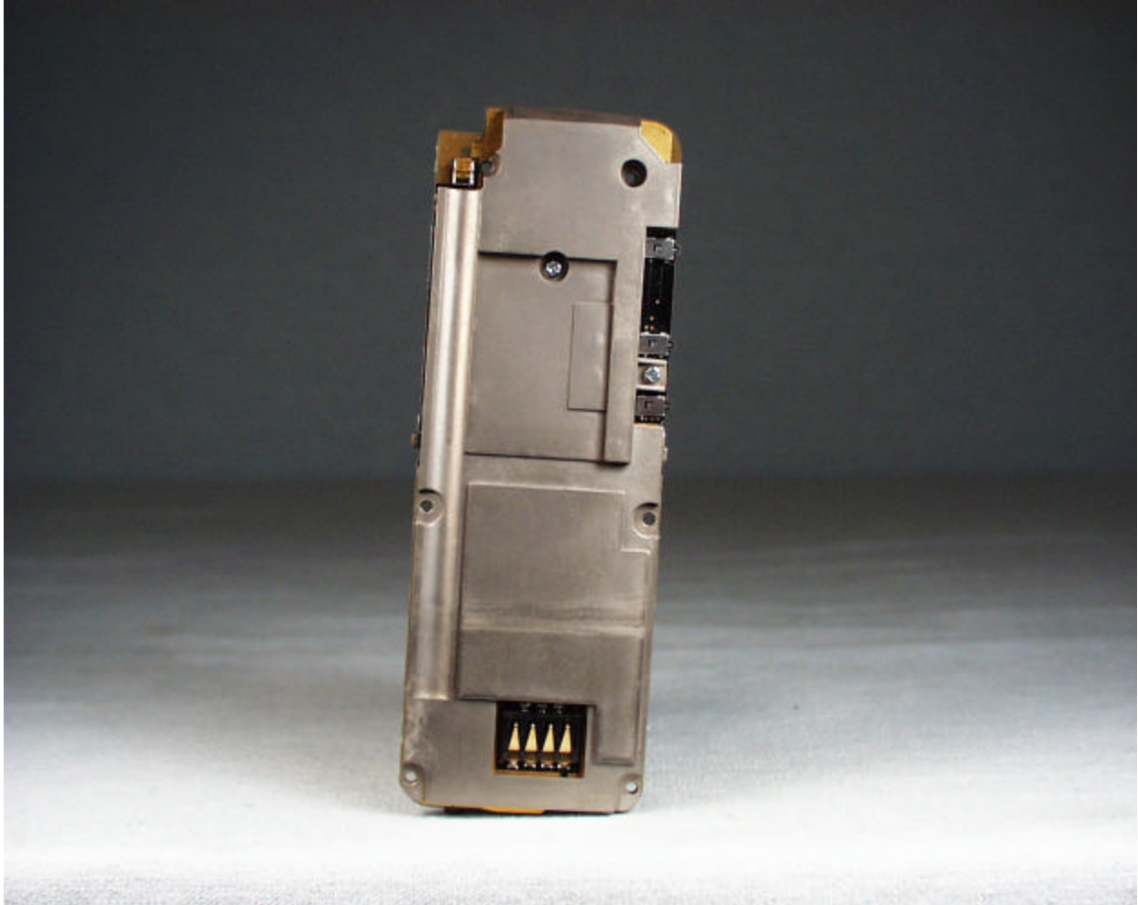
Opposite Side of PCB with Shield Installed (Handset)
