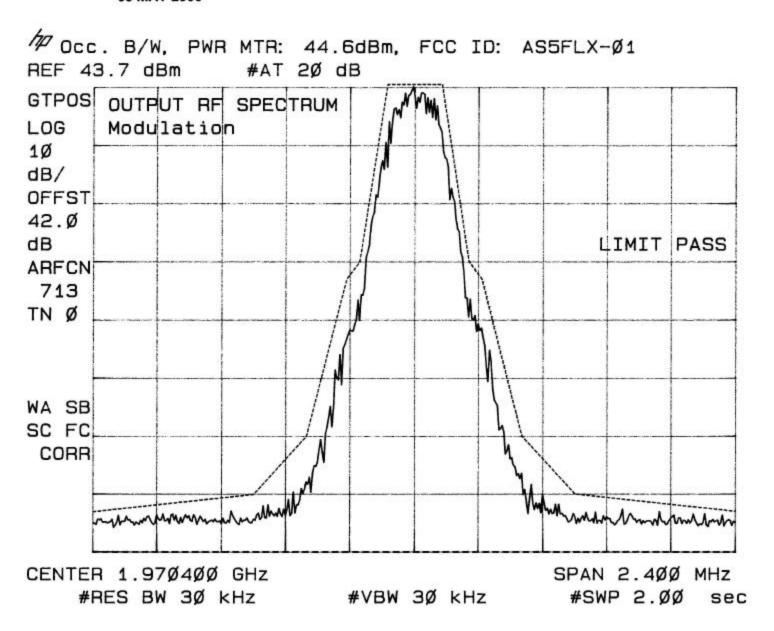
10 Occ. B/W, PWR MTR: 44.6dBm, FCC ID: AS5FLX-Ø1 REF 43.6 dBm #AT 2Ø dB
