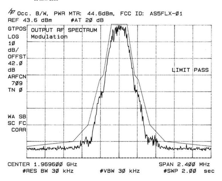
10 Occ. B/W, PWR MTR: 44.6dBm, FCC ID: AS5FLX-Ø1 REF 44.4 dBm #AT 2Ø dB
