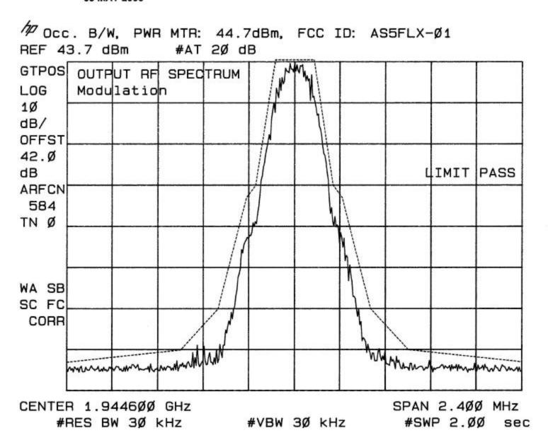
10 Occ. B/W, PWR MTR: 44.7dBm, FCC ID: AS5FLX-Ø1 REF 43.8 dBm #AT 2Ø dB
