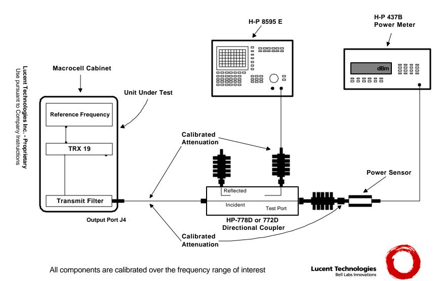
Figure 1B. TEST CONFIGURATION FOR RF POWER OUTPUT
