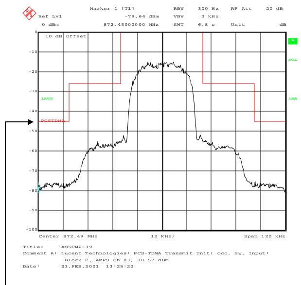
Occupied Bandwidth; Antenna Terminal; Block F; PCS Ch 1335
