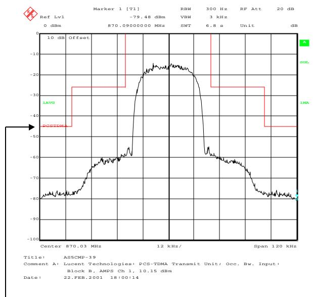
Occupied Bandwidth; Antenna Terminal; Block B; PCS Ch 1164
