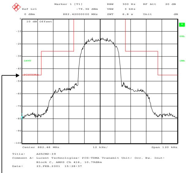
Occupied Bandwidth; Antenna Terminal; Block C; PCS Ch 1502
