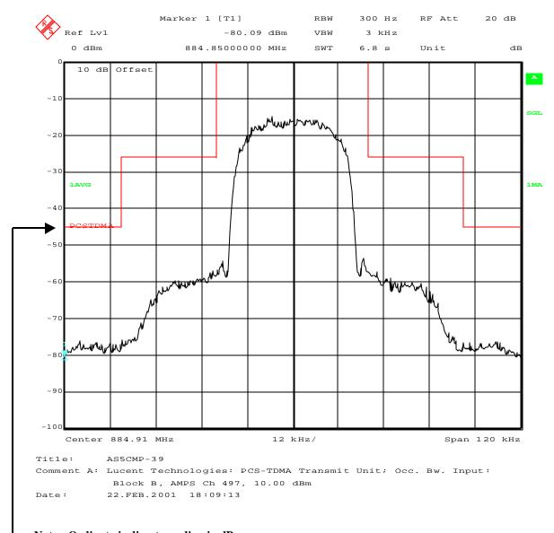
Occupied Bandwidth; Antenna Terminal; Block E; PCS Ch 1250
