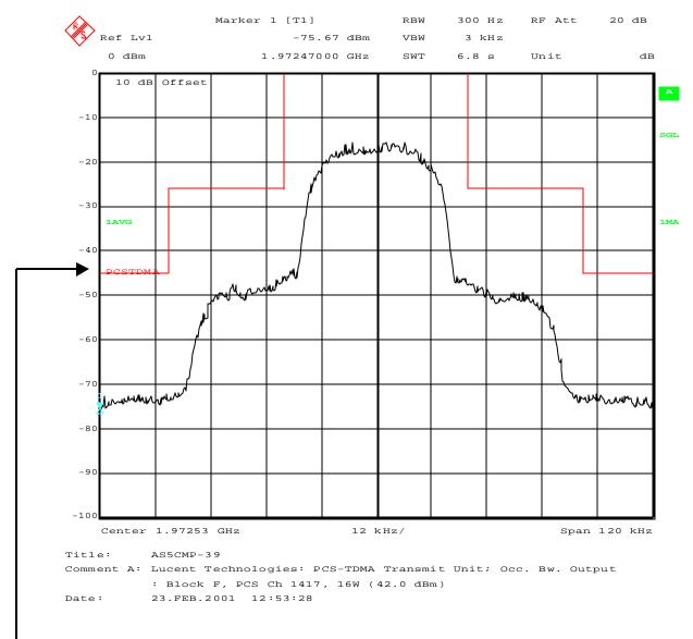
Occupied Bandwidth; Input; Block F; AMPS Ch 83
