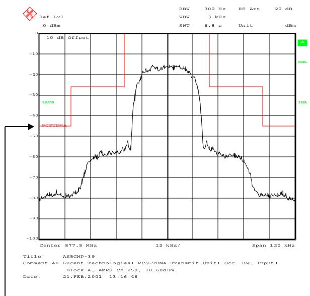
Occupied Bandwidth; Antenna Terminal; Block A; PCS Ch 2
