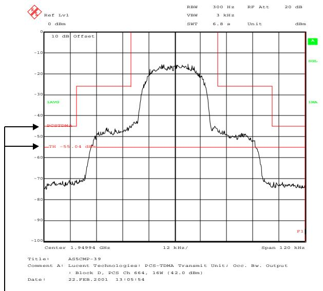
Occupied Bandwidth; Input; Block D; AMPS Ch 664
