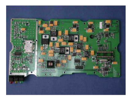
View: Digital Control Circuit Board:- Supply Voltage Power Management and Conversion, Alarm/ Sensor Logic and Synthesizer.
