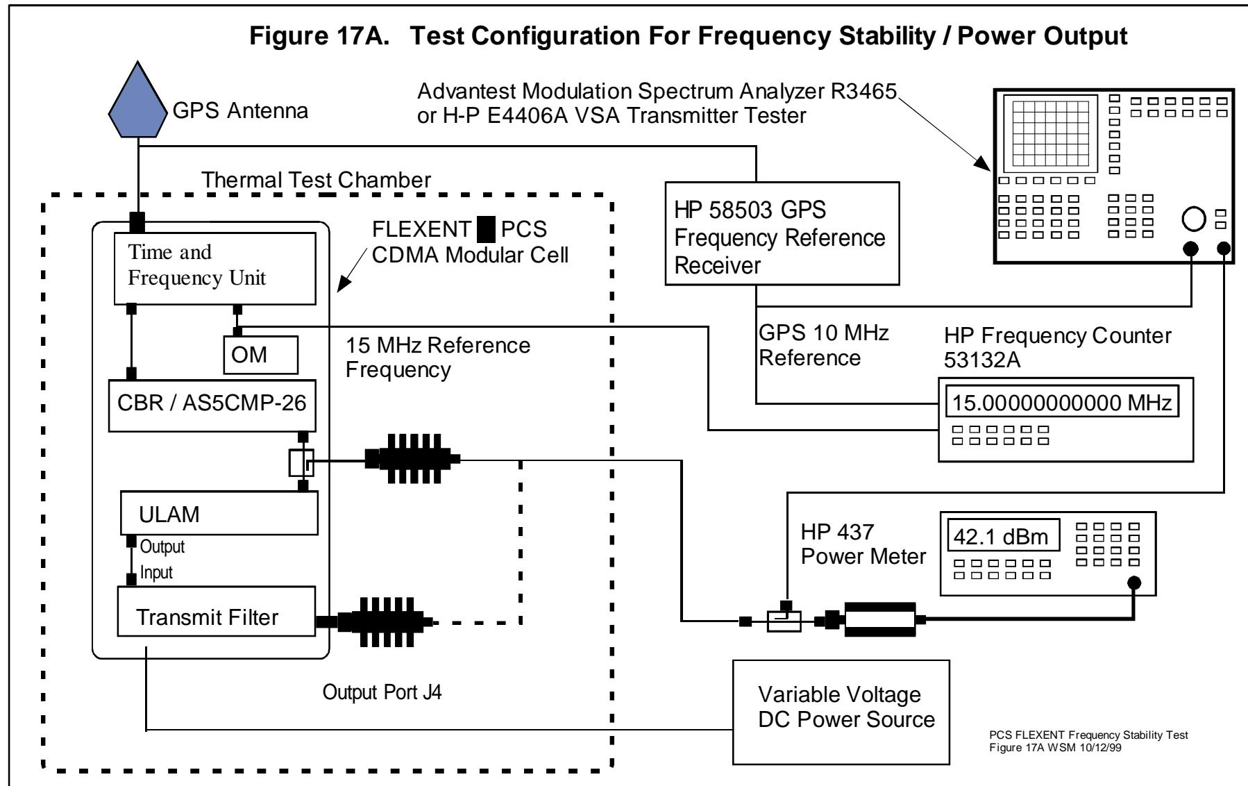
**Exhibit 17: Measurement of Frequency Stability of FLEXENT™ PCS Modular Cell****Exhibit 17: Measurement of Frequency Stability of FLEXENT™ PCS Modular Cell**PCS Sub- Block Tested: B2, PCS Channel 550, 1957.5MHz
