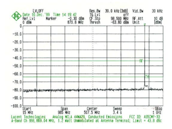
Cellular A-Band Channel 991 869.04 MHz Cellular TDMA/Analog Multi Carrier Linear Amplifier, 44WA29 Output at transmit antenna terminal Plot 1 of 2
