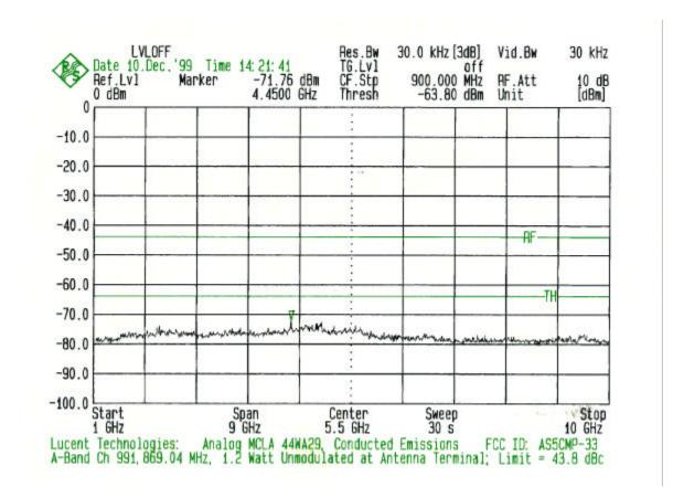
Cellular A-Band Channel 991 869.04 MHz Cellular TDMA/Analog Multi Carrier Linear Amplifier, 44WA29 Output at transmit antenna terminal Plot 2 of 2
