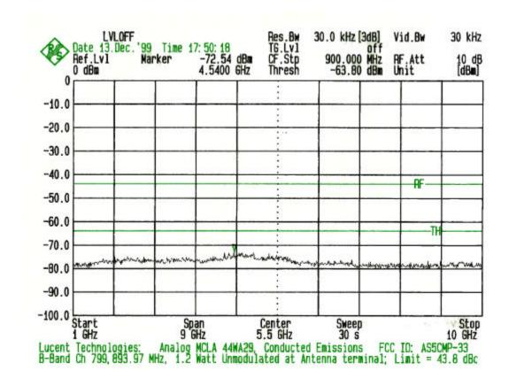
Cellular B-Band Channel 799, 893.97 MHz Cellular TDMA/Analog Multi Carrier Linear Amplifier, 44WA29 Output at transmit antenna terminal
