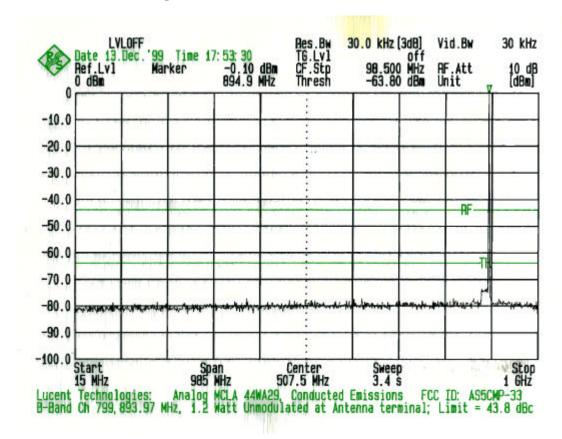
Cellular B-Band Channel 799, 893.97 MHz Cellular TDMA/Analog Multi Carrier Linear Amplifier, 44WA29 Output at transmit antenna terminal
