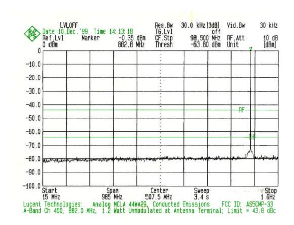
Cellular A-Band Channel 400, 882.00 MHz Cellular TDMA/Analog Multi Carrier Linear Amplifier, 44WA29 Output at transmit antenna terminal Plot 1 of 2
