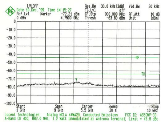
Cellular A-Band Channel 400, 882.00 MHz Cellular TDMA/Analog Multi Carrier Linear Amplifier, 44WA29 Output at transmit antenna terminal
