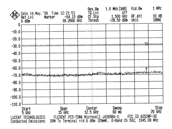
PCS D-Block: Lower Edge Channel Channel 502, 1945.08 MHz
