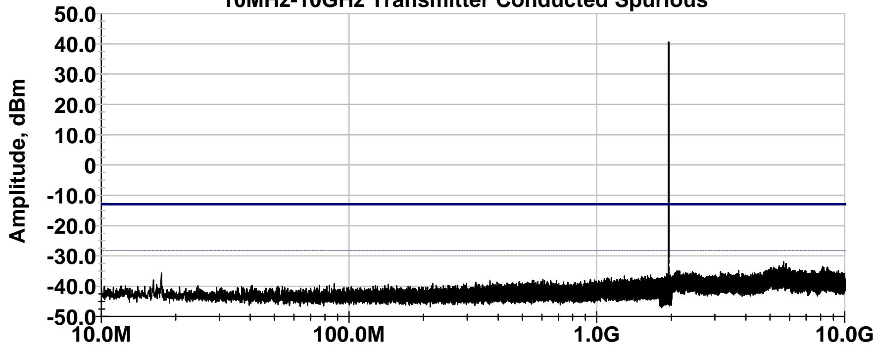
**Frequency, Hz** Flexent PCS CDMA Class B uCell w/ Ascom PS
