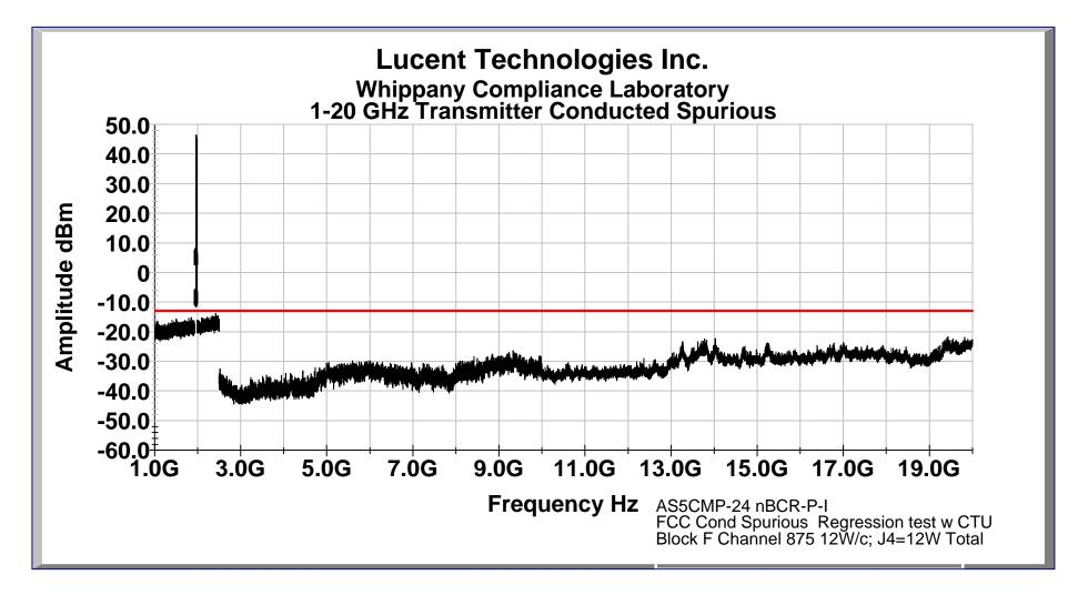
FCC Conducted Spurious: New Lineup BCR w/Panasonic Agile Synthesizer w/ AS5CMP-23 CTU; PCS C Block
