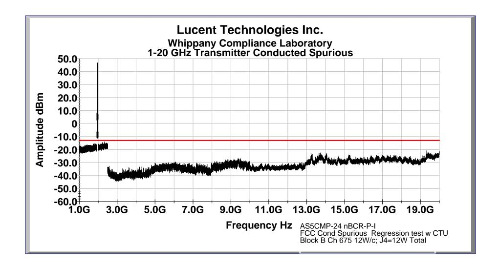
FCC Conducted Spurious: New Lineup BCR w/M/A Com Agile Synthesizer w/ AS5CMP-23 CTU; PCS E Block
