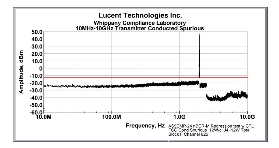
FCC Conducted Spurious: New Lineup BCR w/M/A Com Agile Synthesizer w/ AS5CMP-23 CTU; PCS F Block
