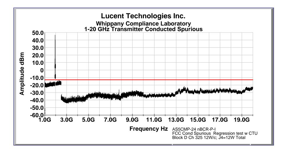
FCC Conducted Spurious: New Lineup BCR w/Panasonic Agile Synthesizer w/ AS5CMP-23 CTU; PCS B Block
