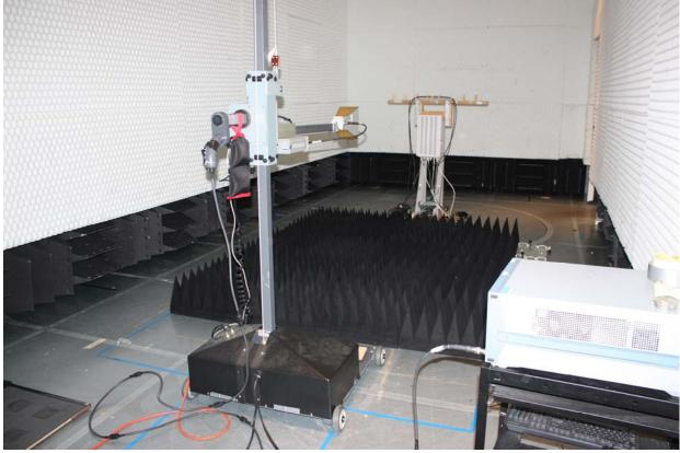
**Radiated Test Setup -Product Configuration**
