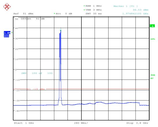
TX Spurious; Test Eng:SG; LTE B25 RRH AR1.0; 1975M:64QAM 1957.5M:QPSK/16QAM; 15+10M BW; BLK B/F; Port 2; 30W Date: 3.0CT.2016 10:24:37
