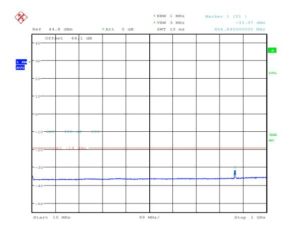
TX Spurious; Test Eng:SG; LTE B25 RRH AR1.0; 1982.5:64QAM 1992.5M:QPSK/16QAM; 5+5M BW; BLK A; Port 3; 30W Date: 27.SEP.2016 14:20:46
