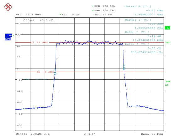
26dB Bandwidth; Test Eng:JY; LTE B25 RRH AR1.0; 1962.5M 16QAM; 15M BW; BLK E; Port 3; 30W; FCC ID-AS5BBTRX-22 Date: 20.SEP.2016 09:03:16
