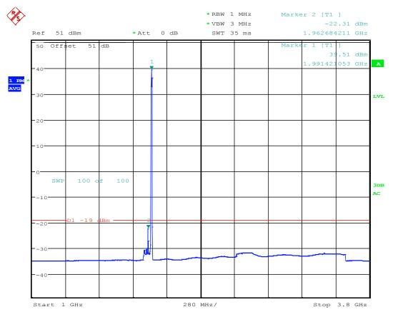
TX Spurious; Test Eng:JY; LTE B25 RRH AR1.0; 1992.5M QPSK; 5M BW; BLK G; Port 3; 30W ; FCC ID-AS5BBTRX-22 Date: 13.SEP.2016 16:51:55
