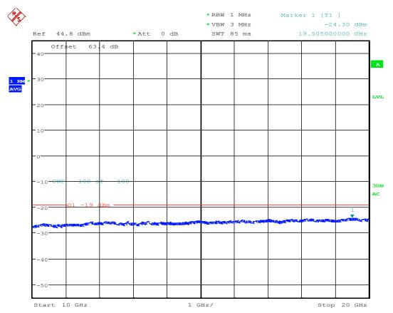
TX Spurious; Test Eng:JY; LTE B25 RRH AR1.0; 1987.5M QPSK; 15M BW; BLK G; Port 3; 30W; HPF; FCC ID-AS5BBTRX-22 Date: 20.SEP.2016 08:28:33
