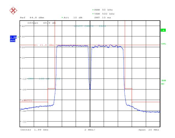
Occupied Bandwidth; Test Eng:SG; LTE B25 RRH AR1.0; 1987.5M: 64QAM 1992.5M:QPSK/16QAM; 5+5M BW; BLK A; Port 4; 30W Date: 27.SEP.2016 09:43:01
