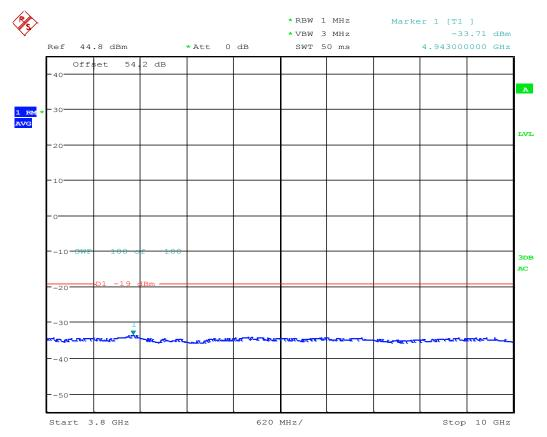
TX Spurious; Test Eng:SG; LTE B25 RRH AR1.0; 1982.5M:64QAM 1992.5M:QPSK/16QAM; 5+5M BW; BLK A; Port 3; 30W ; HPF Date: 27.SEP.2016 14:27:59
