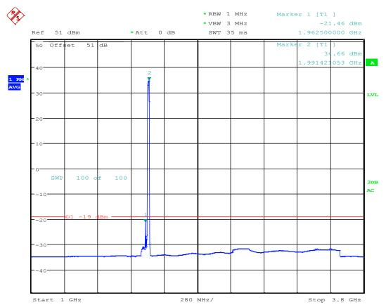
TX Spurious; Test Eng:JY; LTE B25 RRH AR1.0; 1987.5M QPSK; 15M BW; BLK G; Port 3; 30W ; FCC ID-AS5BBTRX-22 Date: 20.SEP.2016 08:24:25
