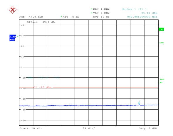
TX Spurious; Test Eng:JY; LTE B25 RRH AR1.0; 1992.5M QPSK; 5M BW; BLK G; Port 3; 30W ; FCC ID-AS5BBTRX-22 Date: 13.SEP.2016 16:50:30
