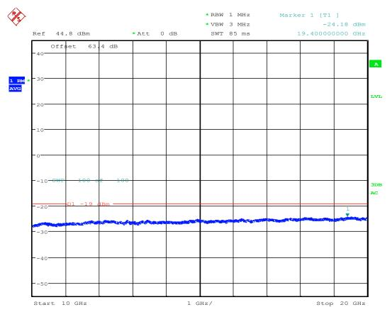
TX Spurious; Test Eng:JY; LTE B25 RRH AR1.0; 1935M QPSK; 10M BW; BLK A; Port 3; 30W ; HPF; FCC ID-AS5BBTRX-22 Date: 14.SEP.2016 11:31:05
