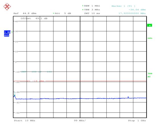
TX Spurious; Test Eng:SG; LTE B25 RRH AR1.0; 1975:64QAM 1957.5M:QPSK/16QAM; 15+10M BW; BLK B/F; Port 2; 30W Date: 3.0CT.2016 10:22:27
