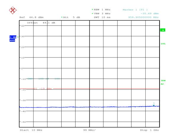
TX Spurious; Test Eng:JY; LTE B25 RRH AR1.0; 1987.5M QPSK; 15M BW; BLK G; Port 3; 30W; FCC ID-AS5BBTRX-22 Date: 20.SEP.2016 08:22:58
