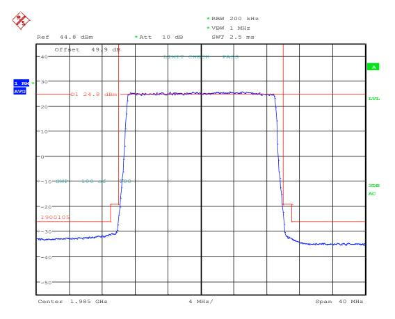
Occupied Bandwidth; Test Eng:JY; LTE B25 RRH AR1.0; 1985M 64QAM; 20M BW; BLK G; Port 3; 30W ; FCC ID-AS5BBTRX-22 Date: 20.SEP.2016 13:08:36
