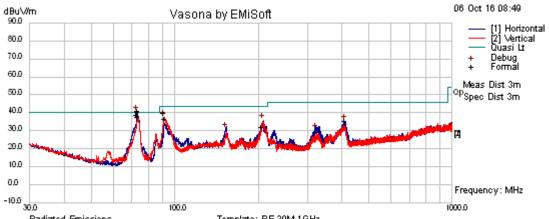
Radiated Emissions Template: RE 30M-1GHz Filename: c:\program files\emisoft - vasona\vesults\2016-120 pos tricarrier -48vdo\RE01 30m-1g FCC B Final.emi
