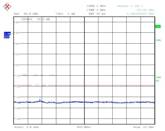
TX Spurious; Test Eng:JY; LTE B25 RRH AR1.0; 1992.5M QPSK; 5M BW; BLK G; Port 3; 30W; HPF; FCC ID-AS5BBTRX-22 Date: 13.SEP.2016 16:53:46
