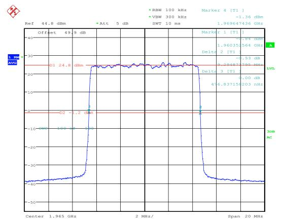
26dB Bandwidth; Test Eng:JY; LTE B25 RRH AR1.0; 1965M 16QAM; 10M BW; BLK E; Port 4; 30W; FCC ID-AS5BBTRX-22 Date: 14.SEP.2016 13:49:54
