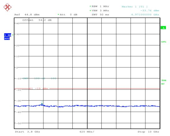
TX Spurious; Test Eng:SG; LTE B25 RRH AR1.0; 1975M:64QAM 1957.5M:QPSK/16QAM; 15+10M BW; BLK B/F; Port 2; 30W ; HPF Date: 3.0CT.2016 10:57:48
