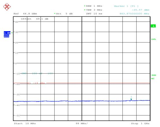
TX Spurious; Test Eng:JY; LTE B25 RRH AR1.0; 1935M QPSK; 10M BW; BLK A; Port 3; 30W ; FCC ID-AS5BBTRX-22 Date: 14.SEP.2016 11:27:42
