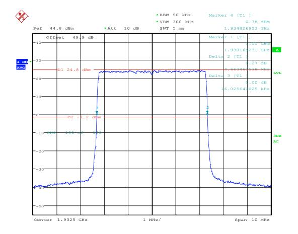
26dB Bandwidth; Test Eng:JY; LTE B25 RRH AR1.0; 1932.5M 64QAM; 5M BW; BLK A; Port 3; 30W ; FCC ID-AS5BBTRX-22 Date: 13.SEP.2016 16:00:28
