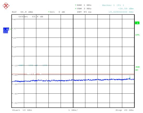
TX Spurious; Test Eng:JY; LTE B25 RRH AR1.0; 1985M
