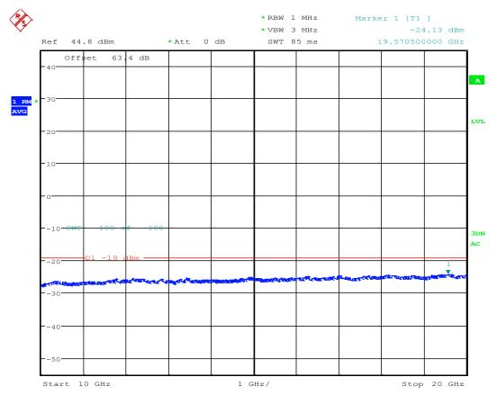
TX Spurious; Test Eng:JY; LTE B25 RRH AR1.0; 1992.5M QPSK; 5M BW; BLK G; Port 3; 30W ; HPF; FCC ID-AS5BBTRX-22 Date: 13.SEP.2016 16:55:04
