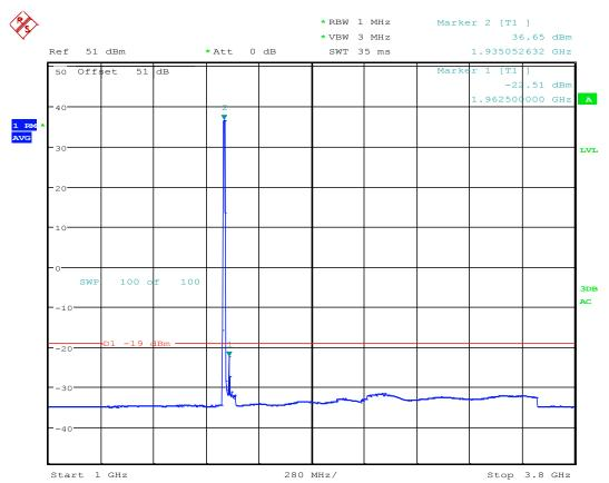
TX Spurious; Test Eng:JY; LTE B25 RRH AR1.0; 1935M QPSK; 10M BW; BLK A; Port 3; 30W ; FCC ID-AS5BBTRX-22 Date: 14.SEP.2016 11:28:29
