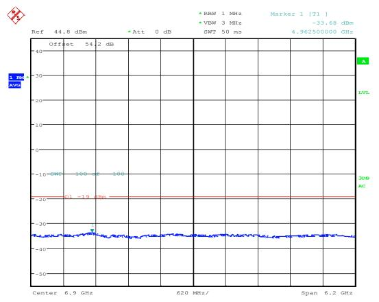
TX Spurious; Test Eng:JY; LTE B25 RRH AR1.0; 1985M 64QAM; 20M BW; BLK G; Port 3; 30W; HPF; FCC ID-AS5BBTRX-22 Date: 20.SEP.2016 13:24:51
