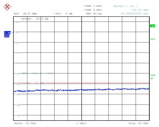
TX Spurious; Test Eng:SG; LTE B25 RRH AR1.0; 1975M:64QAM 1957.5M:QPSK/16QAM; 15+10M BW; BLK B/F; Port 2; 30W ; HPF Date: 3.0CT.2016 11:03:00
