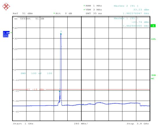
TX Spurious; Test Eng:JY; LTE B25 RRH AR1.0; 1985M 64QAM; 20M BW; BLK G; Port 3; 30W ; FCC ID-AS5BBTRX-22 Date: 20.SEP.2016 13:22:13
