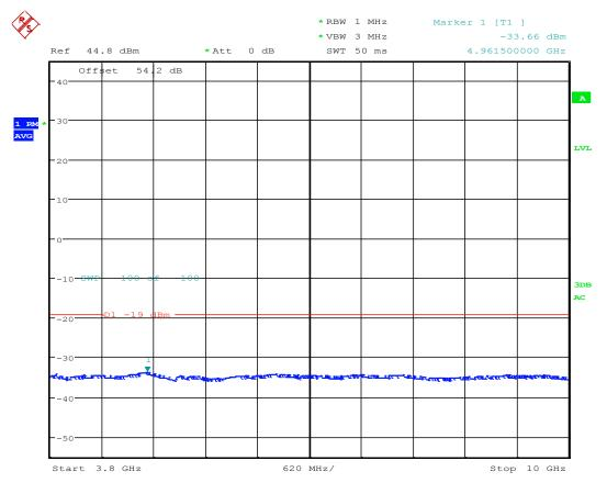
TX Spurious; Test Eng:JY; LTE B25 RRH AR1.0; 1935M QPSK; 10M BW; BLK A; Port 3; 30W ; HPF; FCC ID-AS5BBTRX-22 Date: 14.SEP.2016 11:30:05
