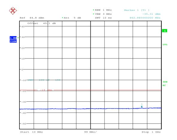
TX Spurious; Test Eng:JY; LTE B25 RRH AR1.0; 1985M 64QAM; 20M BW; BLK G; Port 3; 30W; FCC ID-AS5BBTRX-22 Date: 20.SEP.2016 13:18:27
