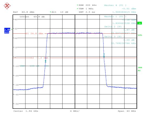
Occupied Bandwidth; Test Eng:JY; LTE B25 RRH AR1.0; 1940M QPSK; 20M BW; BLK A; Port 4; 30W ; FCC ID-AS5BBTRX-22 Date: 20.SEP.2016 11:55:30
