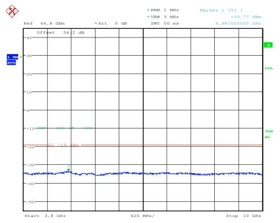
TX Spurious; Test Eng:JY; LTE B25 RRH AR1.0; 1987.5M QPSK; 15M BW; BLK G; Port 3; 30W; HPF; FCC ID-AS5BBTRX-22 Date: 20.SEP.2016 08:36:10
