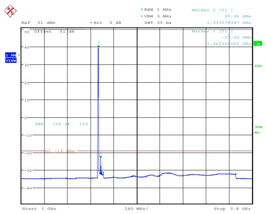
TX Spurious; Test Eng:SG; LTE B25 RRH AR1.0; 1982.5M:64QAM 1992.5M:QPSK/16QAM; 5+5M BW; BLK A; Port 3; 30W Date: 27.SEP.2016 14:23:27
