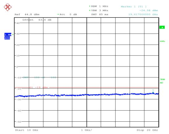
TX Spurious; Test Eng:SG; LTE B25 RRH AR1.0; 1982.5M:64QAM 1992.5M:QPSK/16QAM; 5+5M BW; BLK A; Port 3; 30W ; HPF Date: 27.SEP.2016 14:30:28
