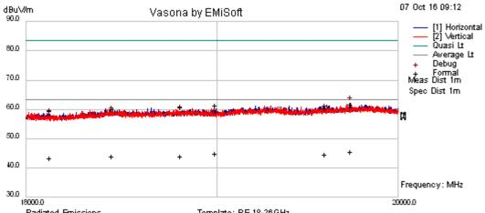
Radiated Emissions Template: RE 18-26GHz Filename: c:\program files\emisoft - vasona\results\2016-120 pos tricarrier -48vdo\T4 RE18g-20GHz FCC B Final.emi
