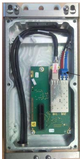
Optical daisy chain Ethernet cable connection (no surge arrester module)
