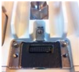
Figure B-4 9764 MCO Wi-Fi AP connection point on 9764 MCO
