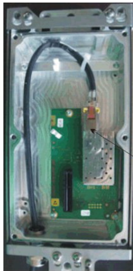
Electrical Backhaul Ethernet cable connection (no surge arrester module)
