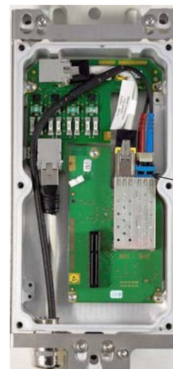
Optical daisy chain Ethernet cable connection (with surge arrester module)
