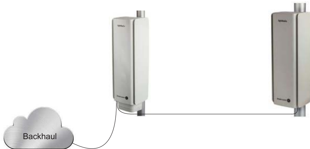
Figure 2-7 9764 MCO daisy chain installation example
