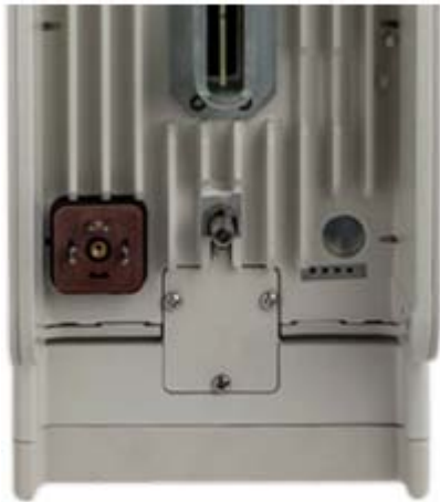
Figure B-14 9764 MCO Wi-Fi AP module attached to 9764 MCO module
