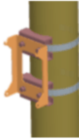
Wall-mount bracket on a large pole
