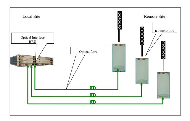
Figure 2 - **B41 RRH8x20-B** System Overview (Star Configuration Supported From BBU)
